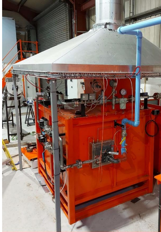
Figure 2. Burner test kiln constructed by Therser UK
