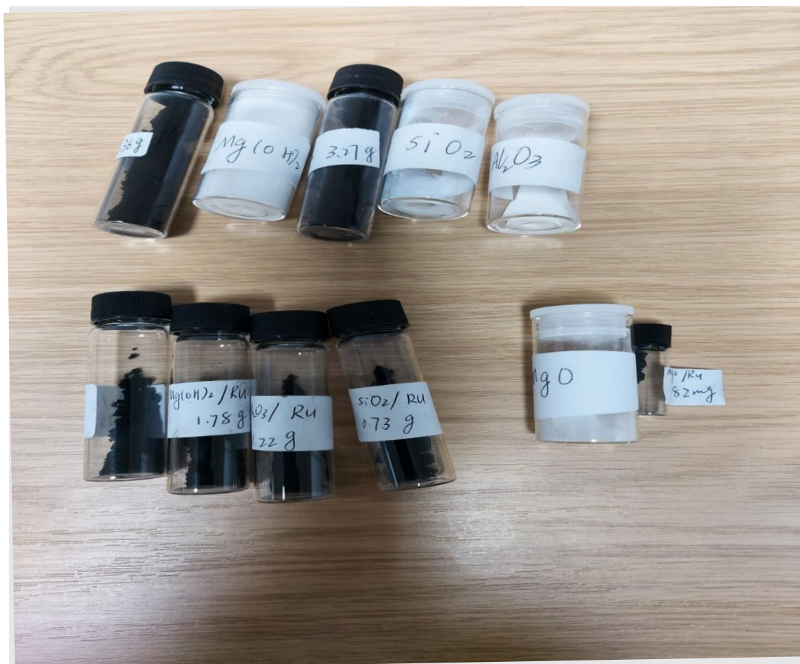
Figure 1: Ruthenium based Ammonia Synthesis catalyst materials
