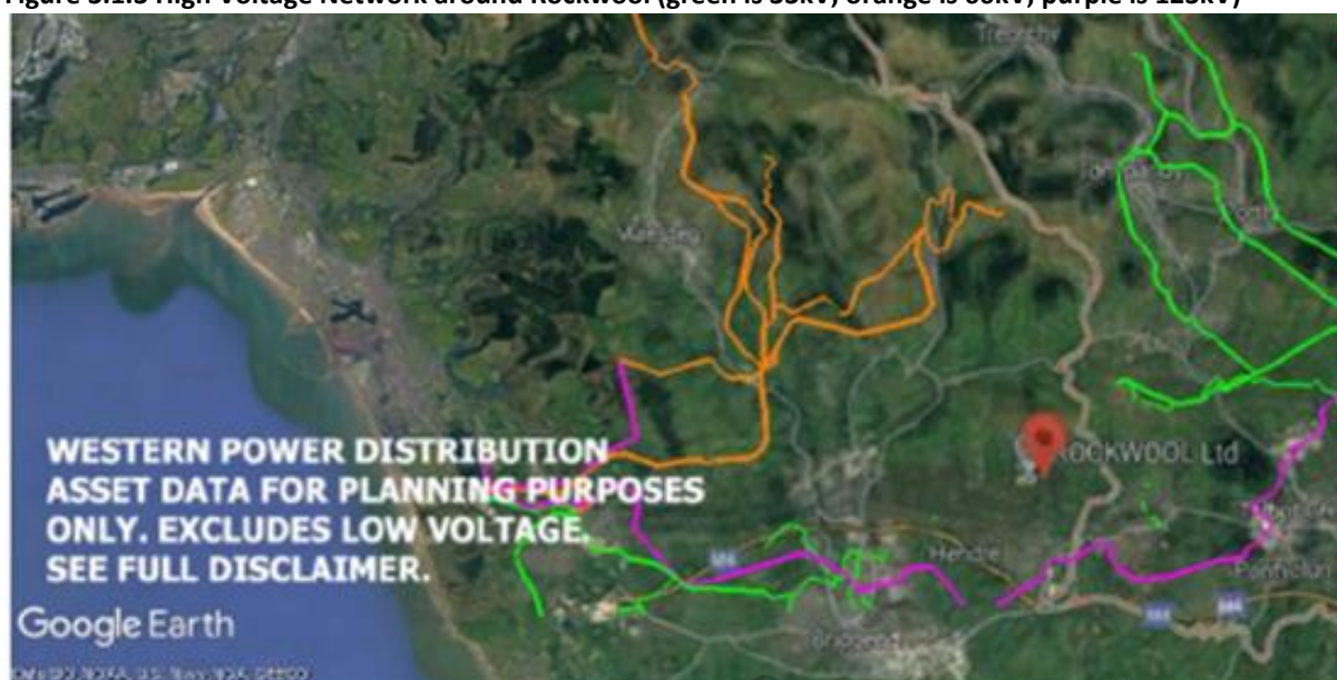
Figure 3.1.3 High Voltage Network around Rockwool (green is 33kV; orange is 66kV; purple is 123kV)
