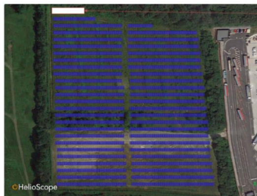
Figure 3.1.5 Initial Solar PV Design, panel rows in blue, electrical substation in white
