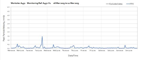
Note: High vibration levels measured at 17:00 on Tuesday 7th March was due to topsoil stripping and pond perimeter works in the vicinity of the monitor.
