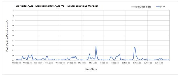
Note: High vibration levels measured at 15:00 on Thursday 16th March was due to topsoil stripping and pond perimeter works in the vicinity of the monitor.
