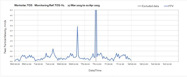
Note: High vibration levels measured at 16:00 on Wednesday 29<sup>th</sup> March were due to excavation, stoning up and ground compaction works taking place close to monitoring station.
