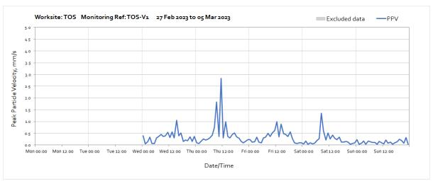
Note: High vibration levels measured at 11:00 on Thursday 2<sup>nd</sup> March were due to the assembly of tunnel boring machine undertaken within 20 meters from the monitoring station.
