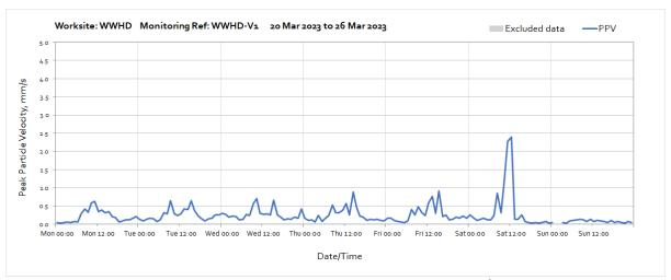
Note: High vibration levels measured between 10:00 and 13:00 on Saturday 25<sup>th</sup> March were due to wagons passing close to the monitoring station. Missing data between 01:00 and 03:00 on Sunday 26<sup>th</sup> March was due to a monitor time adjustment at the start of British Summer Time.
