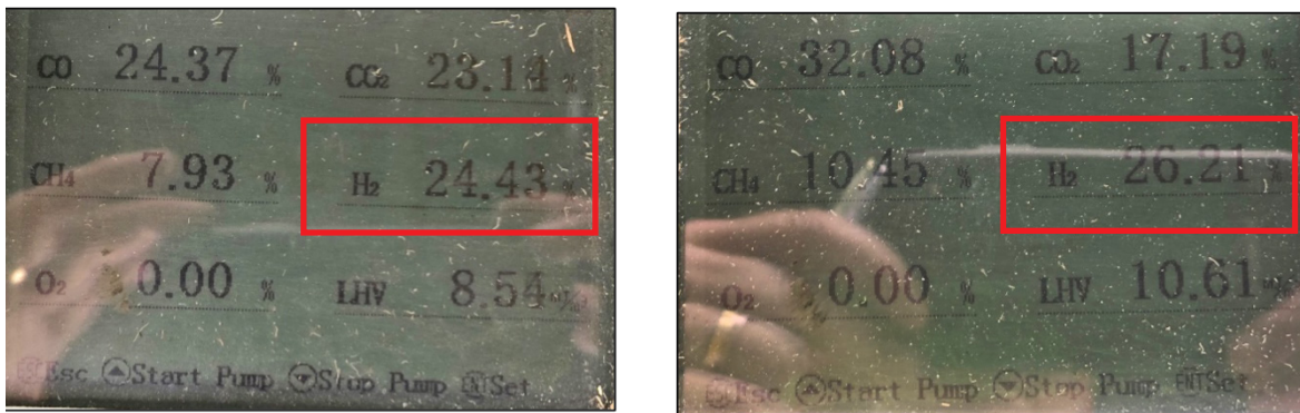
Figure 6 Syngas composition analysis with O 2 air enrichment at 60% (Left 24.43) and 65% (Right 26.21).
