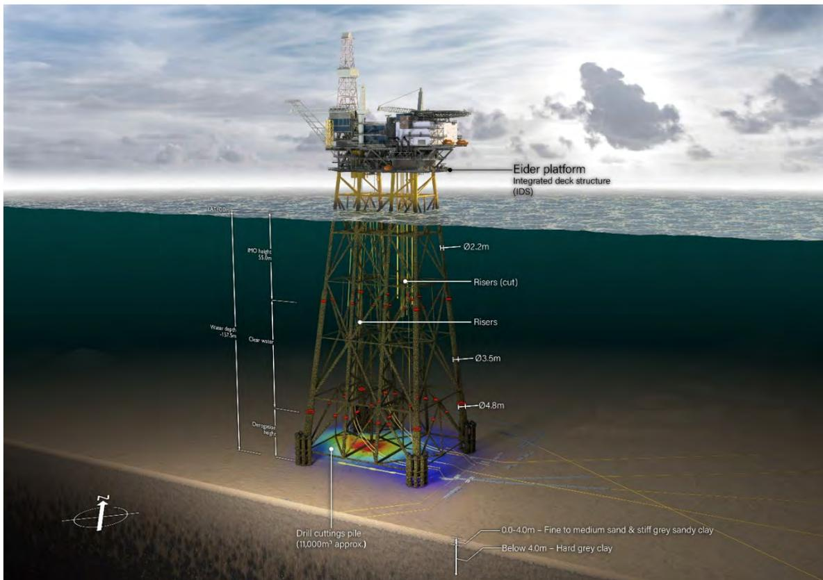
**Figure 2-2 Eider decommissioning schematic**
