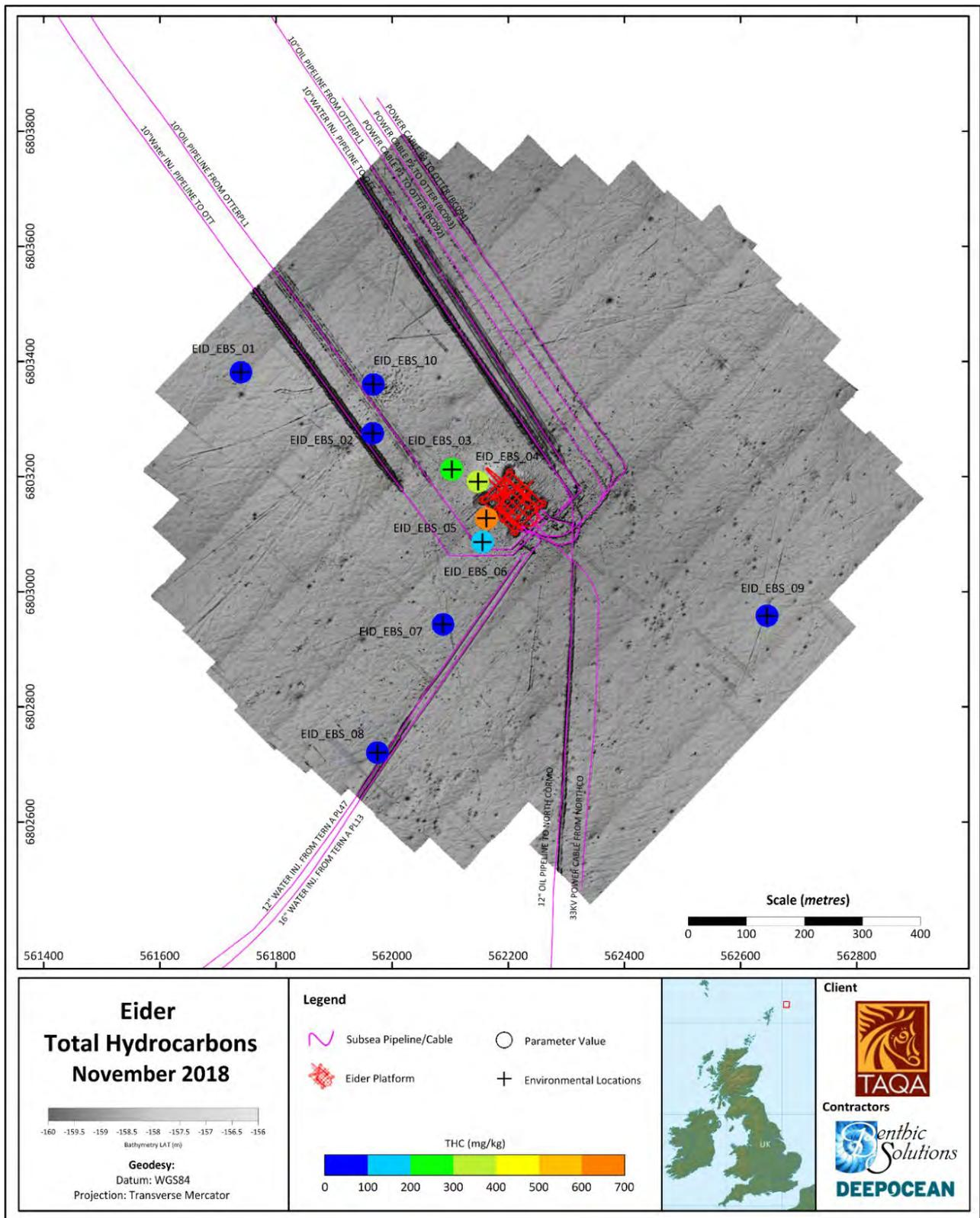
Figure 3-5 Total Hydrocarbon content (THC) around the Eider platform. Benthic Solutions (2019) survey
