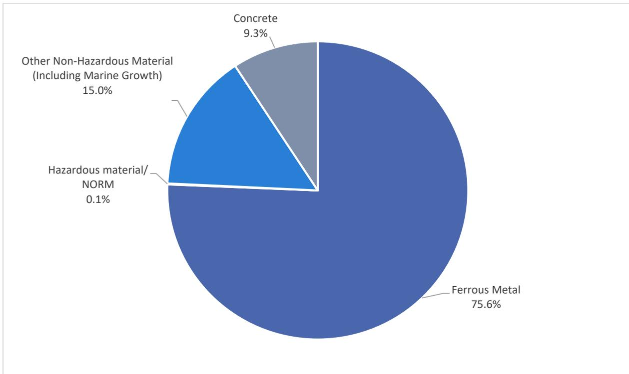
**Figure 2-4 Bulk materials from the Eider Upper Jacket**
