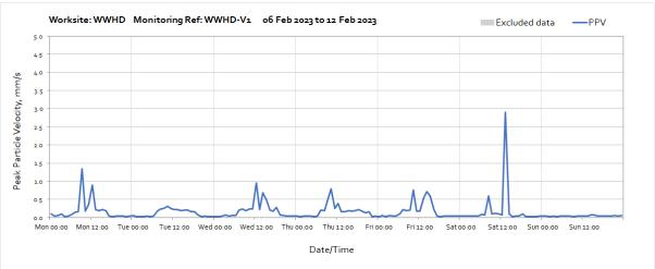
Note: High vibration levels measured at 13:00 on Saturday 11<sup>th</sup> February were due to movement of plant on haul road close to monitoring station.
