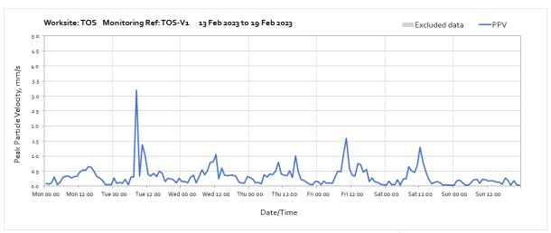
Note: High vibration levels measured between 08:00 and 11:00 on Tuesday 14<sup>th</sup> were due to delivery and assembly of tunnel boring machine undertaken within 20 meters from the monitoring station.
