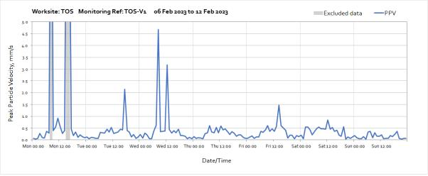
Note: High vibration levels measured at 08:00 and 12:00 on Wednesday 8<sup>th</sup> February were due to delivery and assembly of tunnel boring machine undertaken within 20 meters from the monitoring station.
