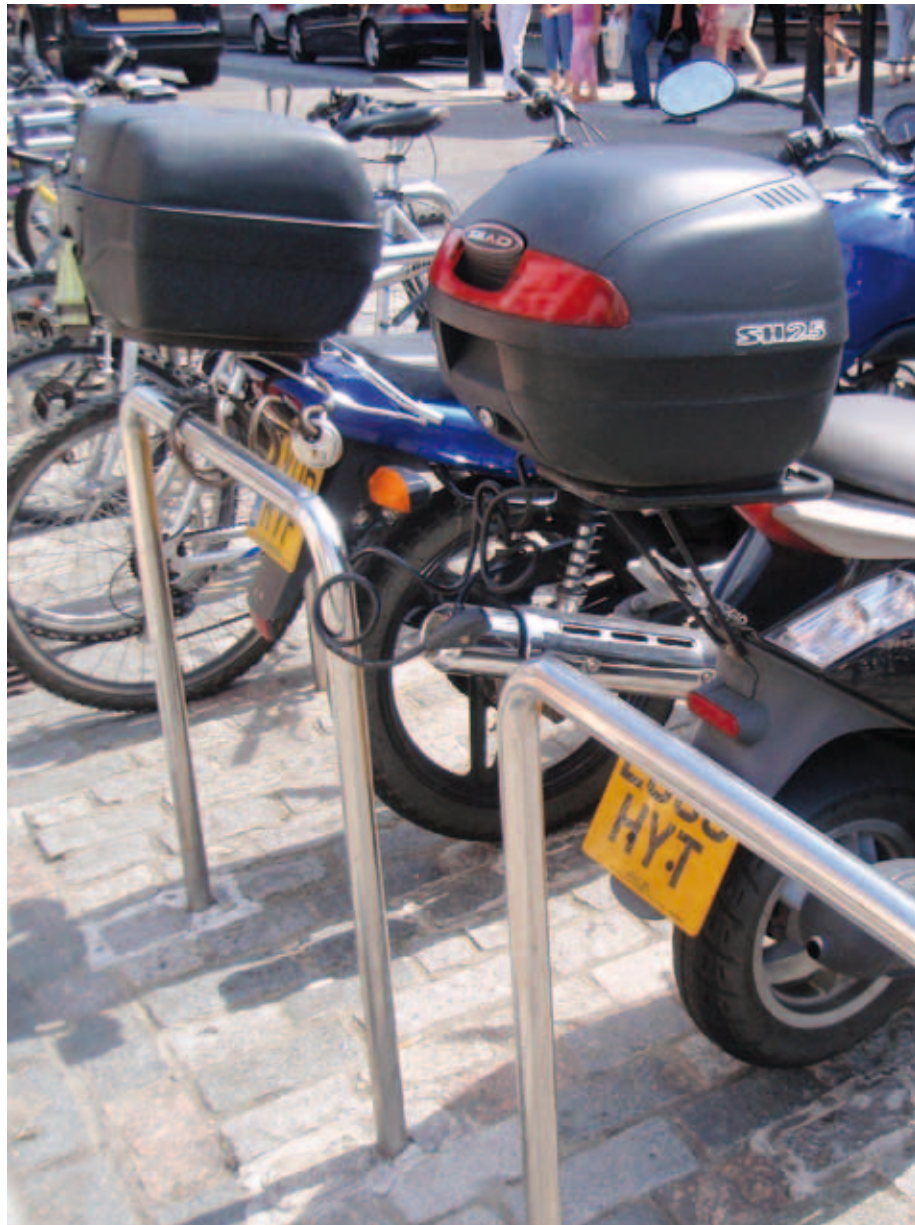
Note, cobbles are not appropriate surface treatment for PTW parking
