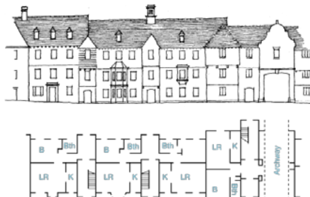
(Top) Front elevation. (Bottom) Ground-floor plan.
