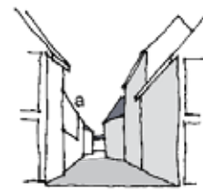
(Top)- Width of space equal to or less than height of enclosing planes. (Bottom) Drop in height at (a) compensated by rise in height on opposite side
