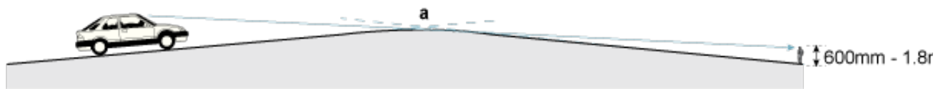
Forward visibility 25m in 20mph (30kph) zones; 43m on 30mph (50kph) roads a. Vertical curve at summit
