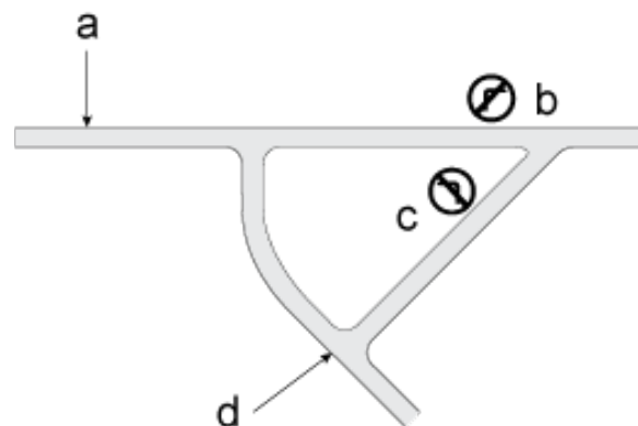
a. 45° b. 'No right turn ahead, turn right here for Road X' sign c. 'No right turn' sign d. 'No left turn' sign e. 'No left turn in Road X, straight on for Road Y' sign
