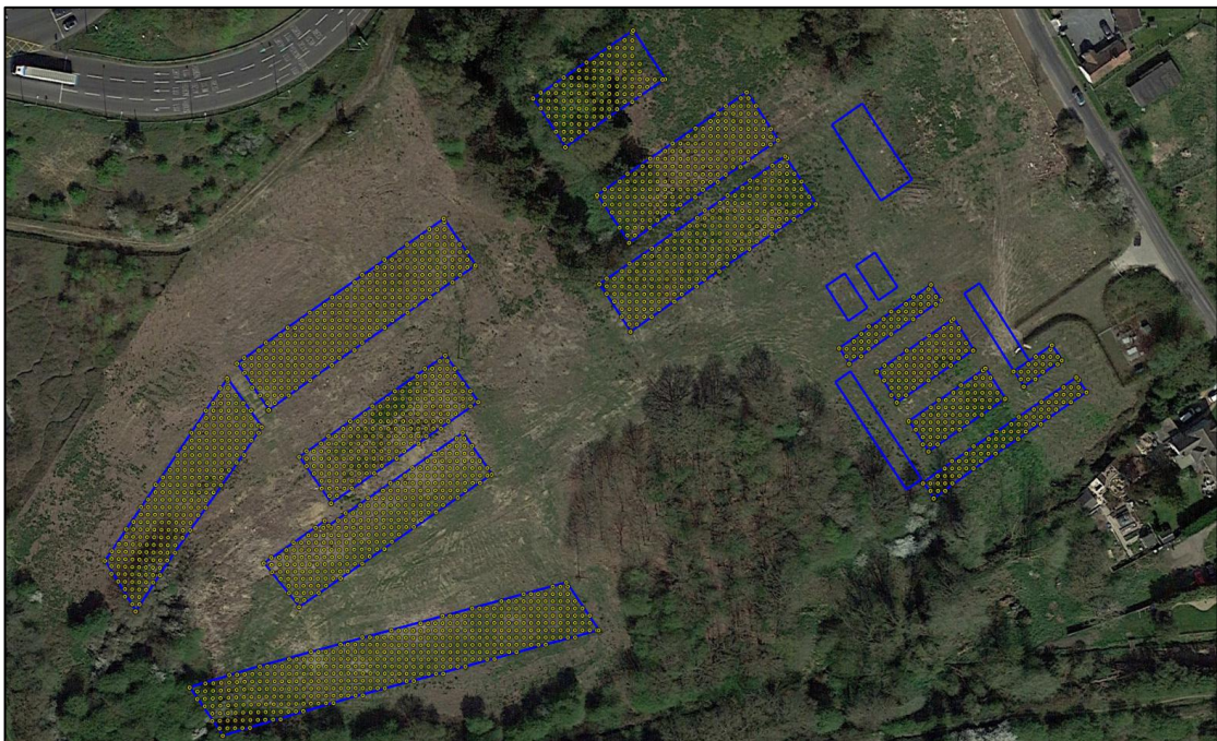
Figure 15 Reflecting areas 11 (yellow radial icons) – Pager Power modelling results for ATC Tower
