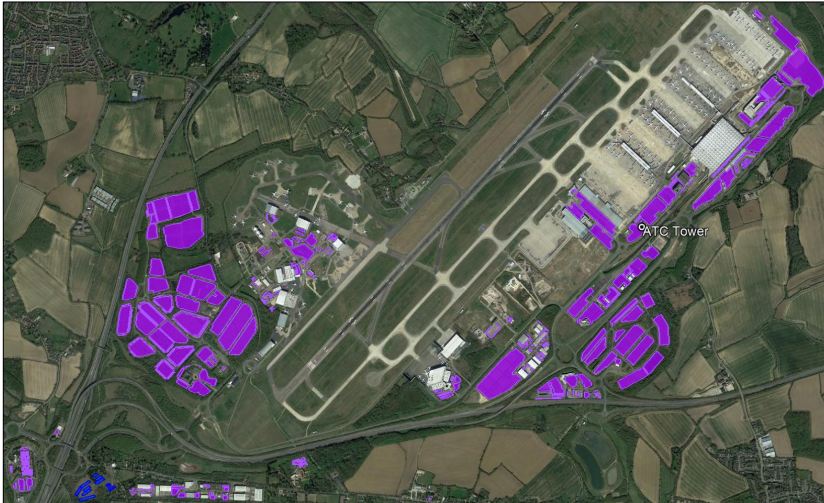
Figure 17 Vehicle parking spaces (purple areas) with the potential to cause solar reflections towards the ATC tower and reflecting areas within the proposed development
