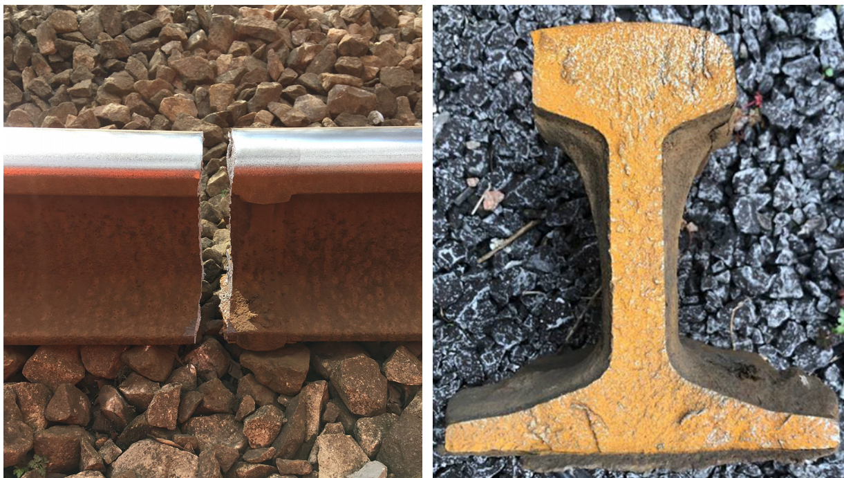
Figure 8: The rail break at Pencoed, in-situ (left-hand image) and its fracture face (right-hand image) (photos courtesy of Network Rail).
