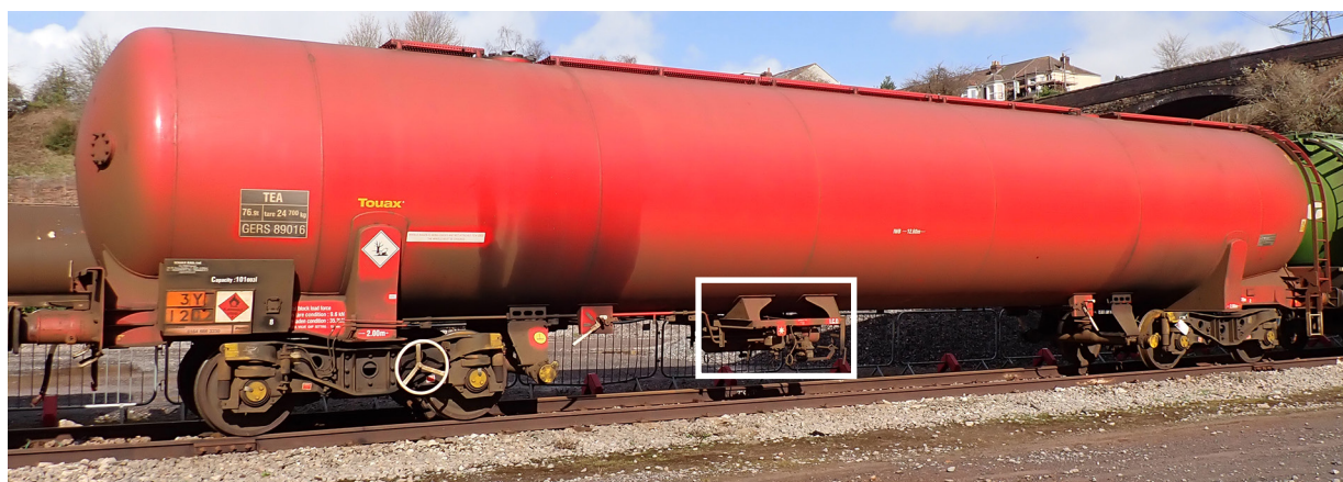
Figure 5: Wagon GERS89016 and its brake group (auxiliary reservoir hidden by brake group).
