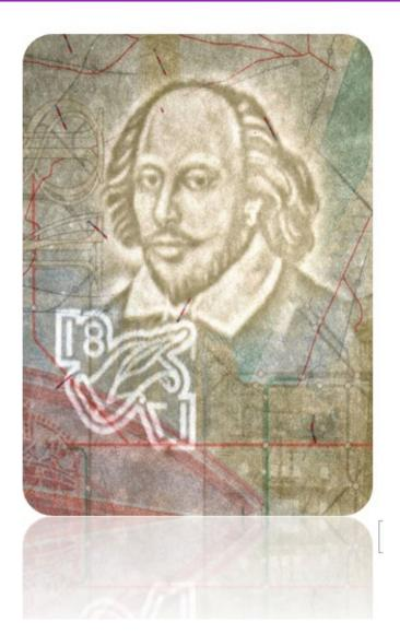
A watermark is created during the paper manufacturing process by varying the thickness of the paper. It is best viewed using **transmitted light** (e.g. holding the paper up to a lamp or by shining a torch light through the paper). A real watermark should usually consist of subtle changes in tone and both lighter and darker areas.
