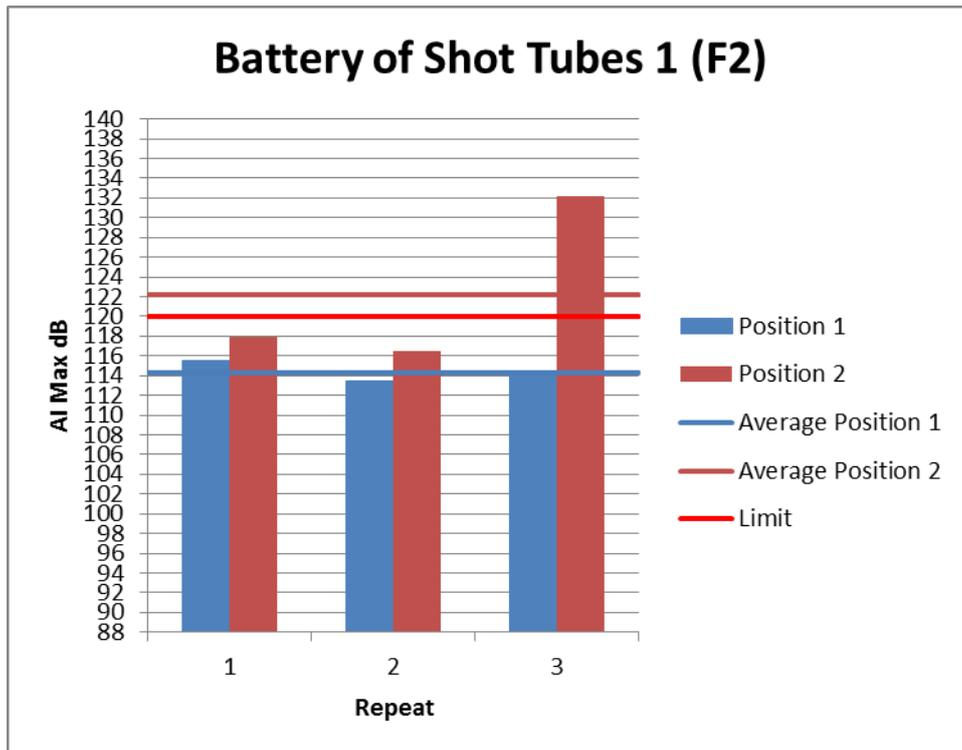
Figure 28: Individual Noise Levels for Battery of Shot Tubes 1 (F2)
