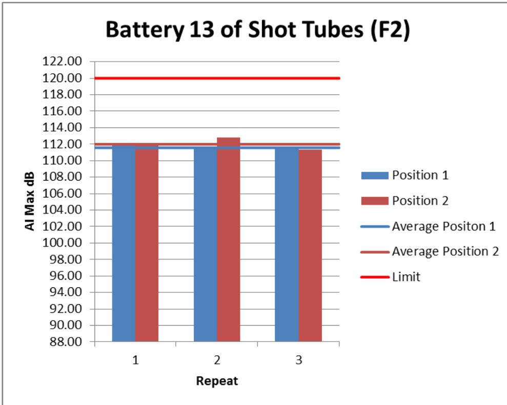
Figure 40: Individual Noise Levels for Battery of Shot Tubes 13 (F2)
