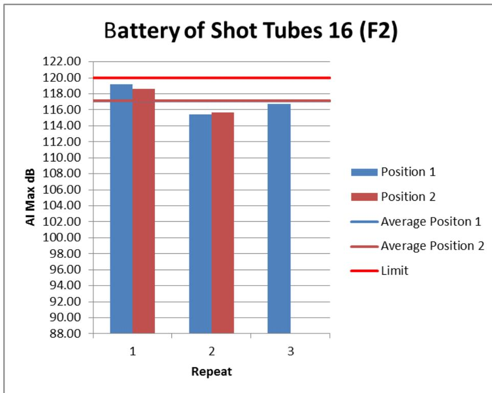
Figure 43: Individual Noise Levels for Battery of Shot Tubes 16 (F2)
