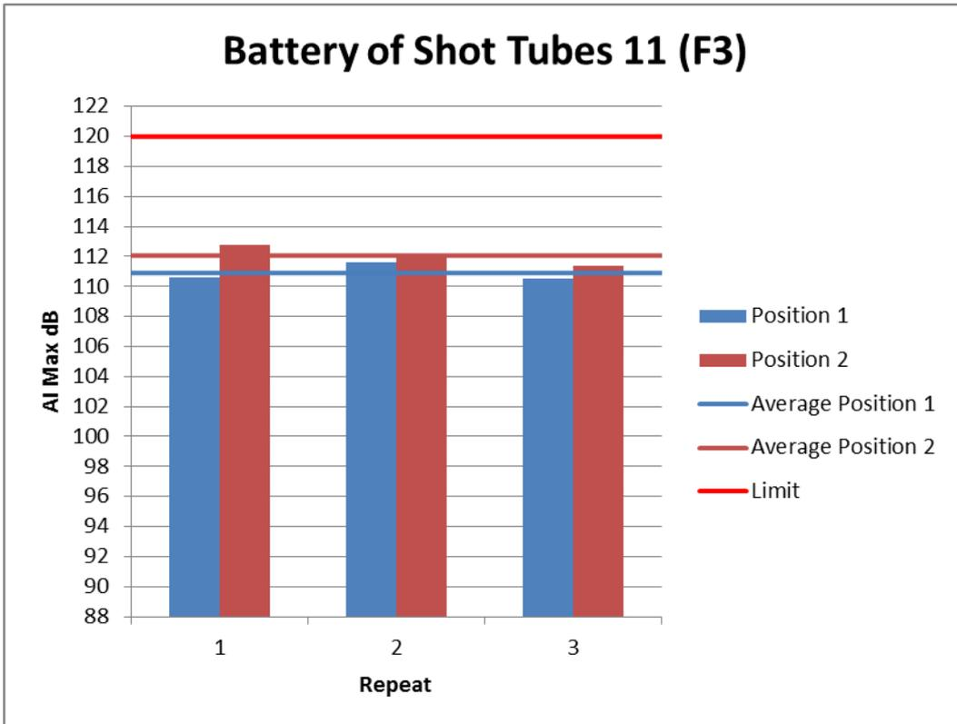
Figure 38: Individual Noise Levels for Battery of Shot Tubes 11 (F3)
