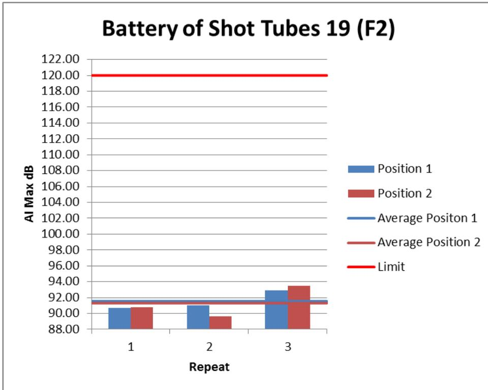
Figure 46: Individual Noise Levels for Battery of Shot Tubes 19 (F2)
