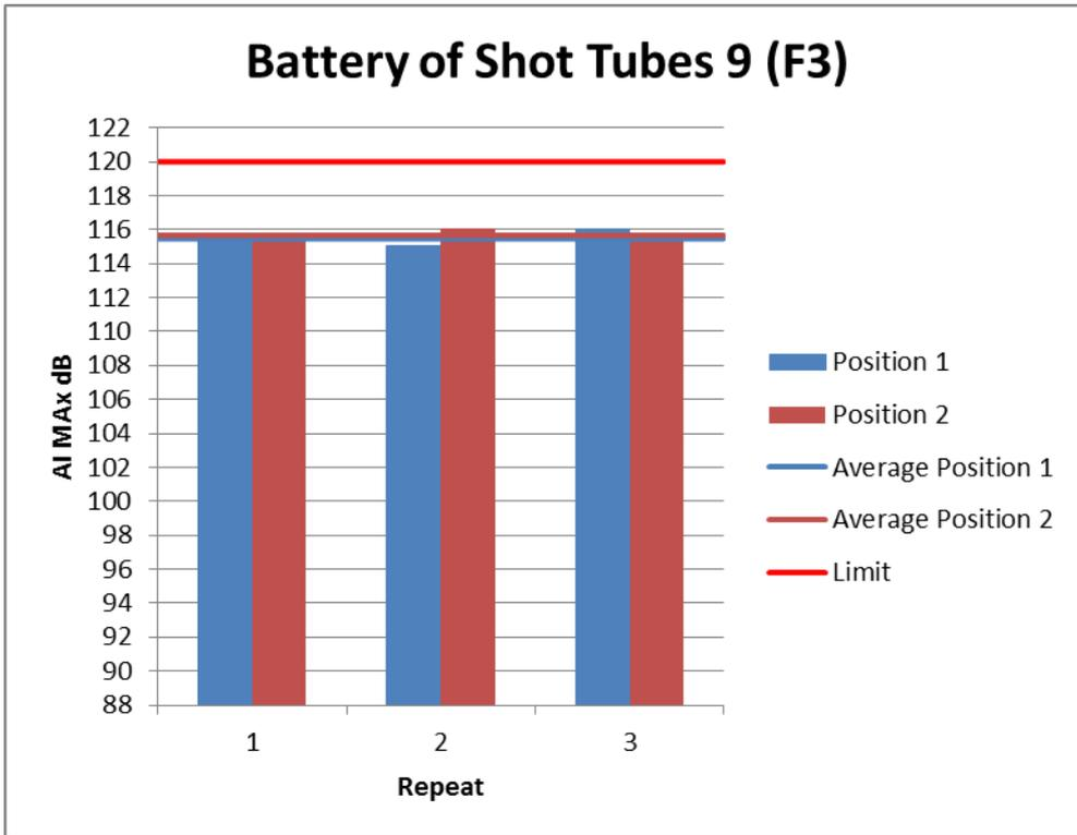
Figure 36: Individual Noise Levels for Battery of Shot Tubes 9 (F3)
