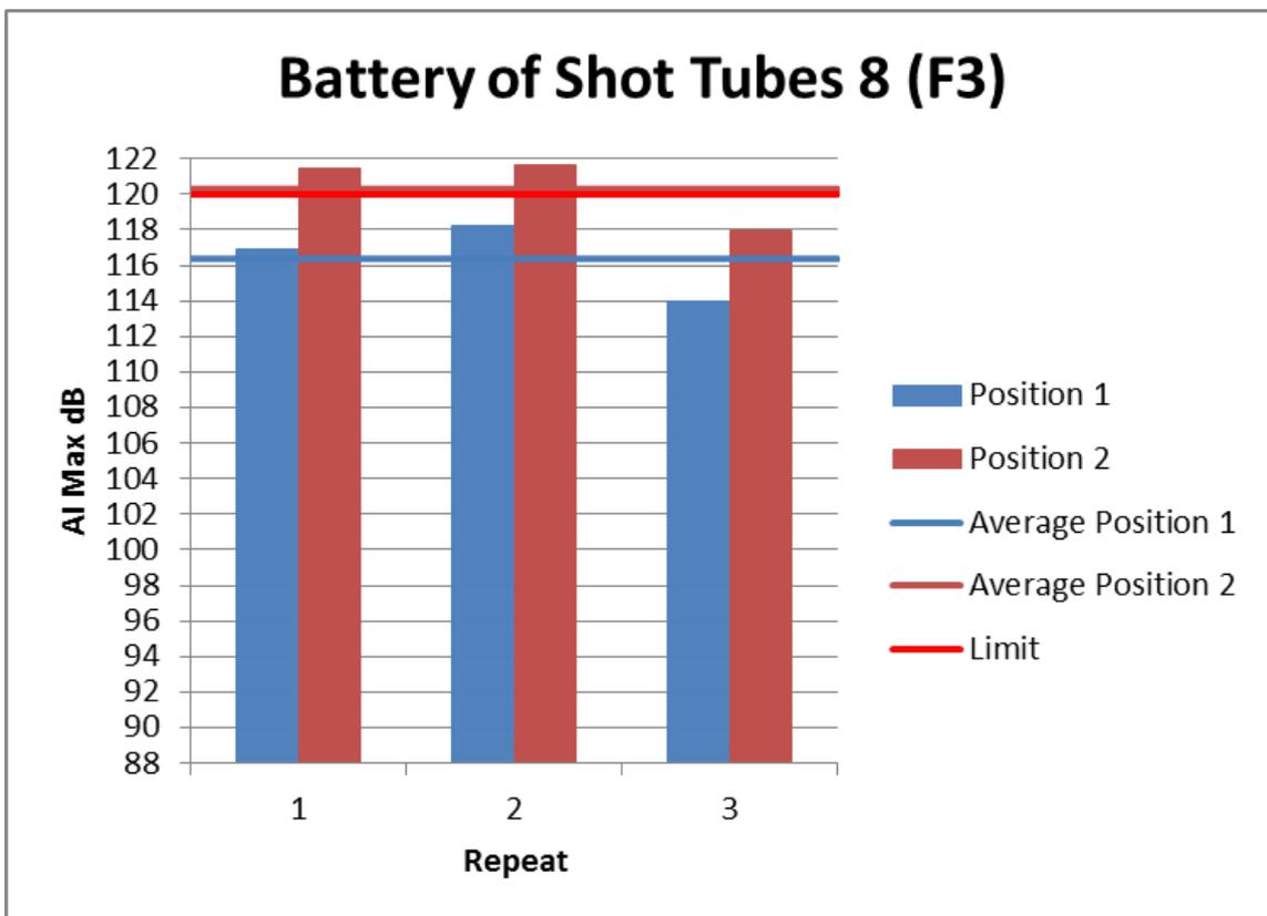
Figure 35: Individual Noise Levels for Battery of Shot Tubes 8 (F3)
