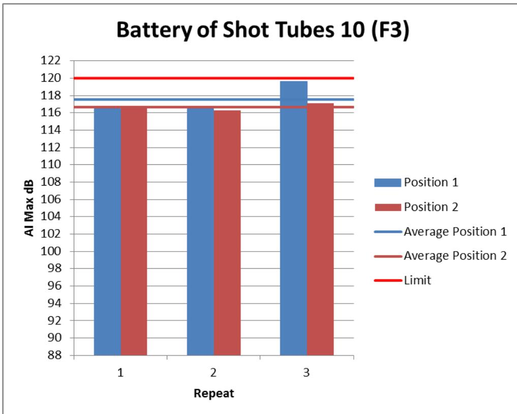
Figure 37: Individual Noise Levels for Battery of Shot Tubes 10 (F3)
