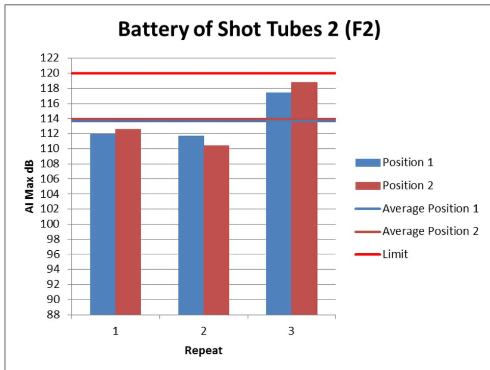
Figure 29: Individual Noise Levels for Battery of Shot Tubes 2 (F2)
