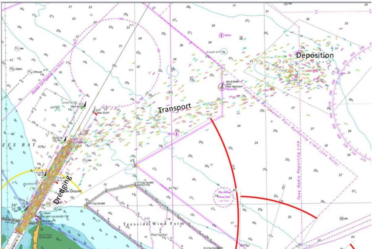
**Fig 9: Compilation of the positions of the dredger over the period 25 September to 4 October every few minutes based on transmissions of its position using the AIS system. Dredging activity in the south-west and deposition site in the north-east.**
