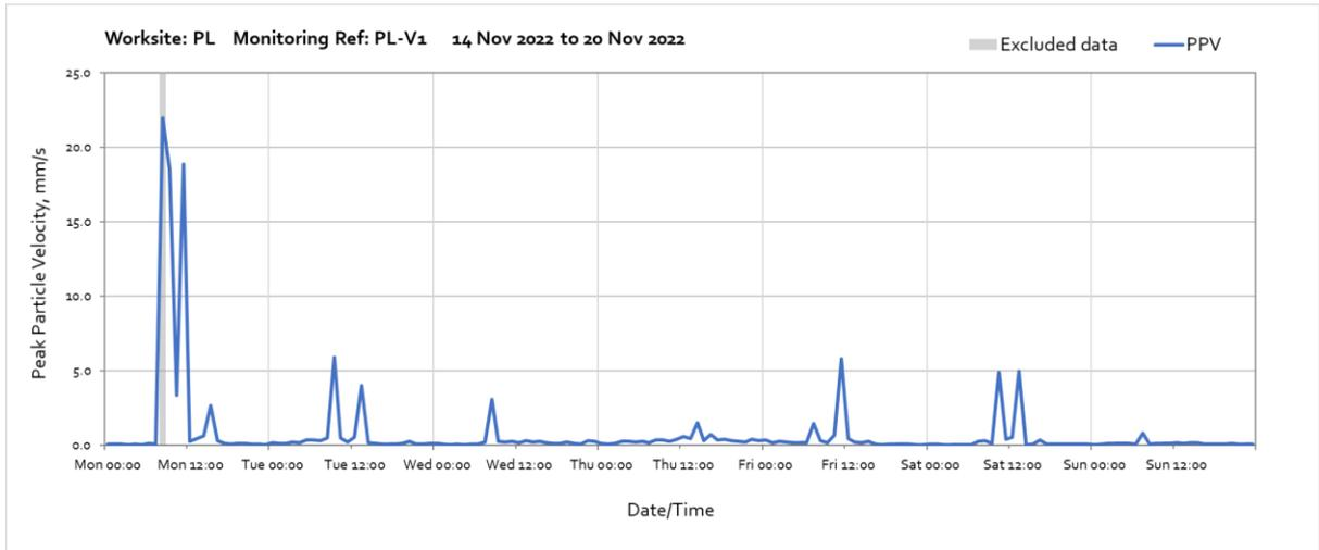
Note: High vibration levels measured at 09:00 on Monday 14<sup>th</sup> November was due to topsoiling and hydroseeding works undertaken in vicinity of the monitor.
