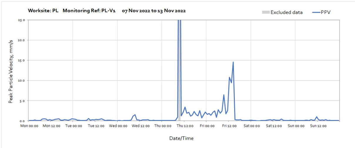
Note: High vibration levels measured between 12:00 to 14:00 on Friday 11<sup>th</sup> November was due to topsoiling and hydroseeding works undertaken in vicinity of the monitor.
