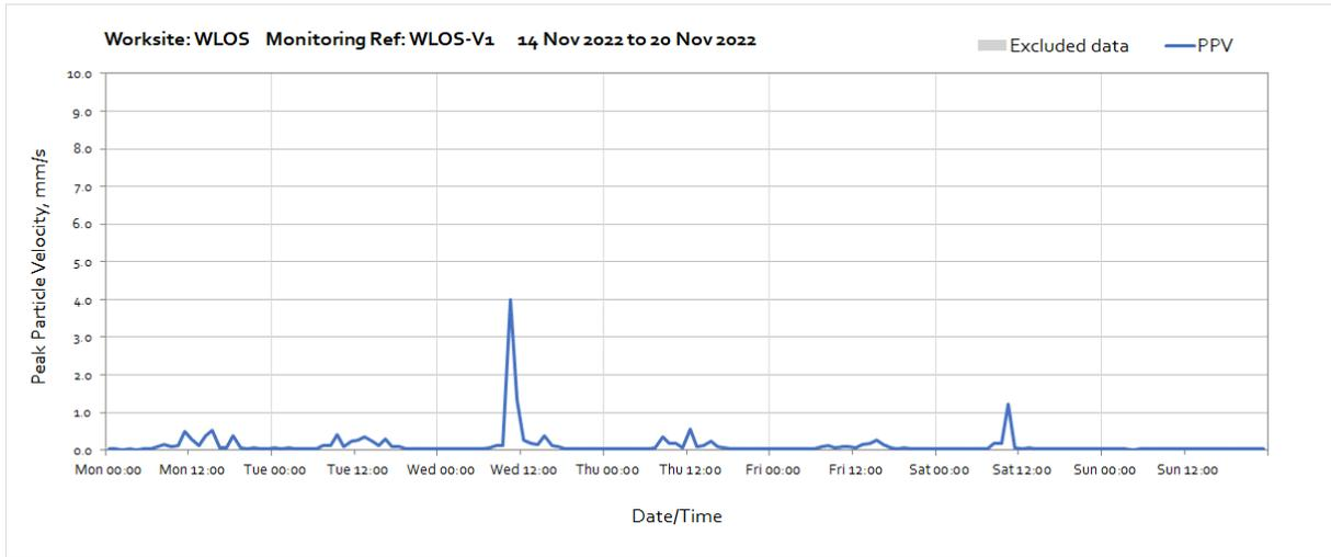
Note: High vibration levels measured at 10:00 on Wednesday 16<sup>th</sup> November was due to ground works undertaken in vicinity of the monitor.
