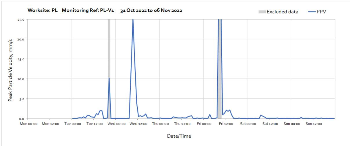
Note: High vibration levels measured at 09:00 on Wednesday 2<sup>nd</sup> November was due to topsoiling and hydroseeding works undertaken in vicinity of the monitor.
