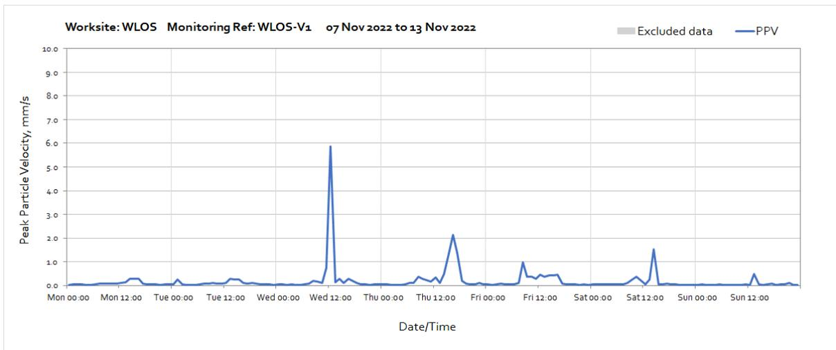
Note: High vibration levels measured at 12:00 on Wednesday 9<sup>th</sup> November was due to ground works undertaken in vicinity of the monitor.
