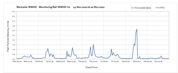
Note: High vibration levels recorded at 12:00 on Saturday 19<sup>th</sup> November were due to pedestrian walkway works using excavators and rollers undertaken 40 meters away from the vibration monitor.
