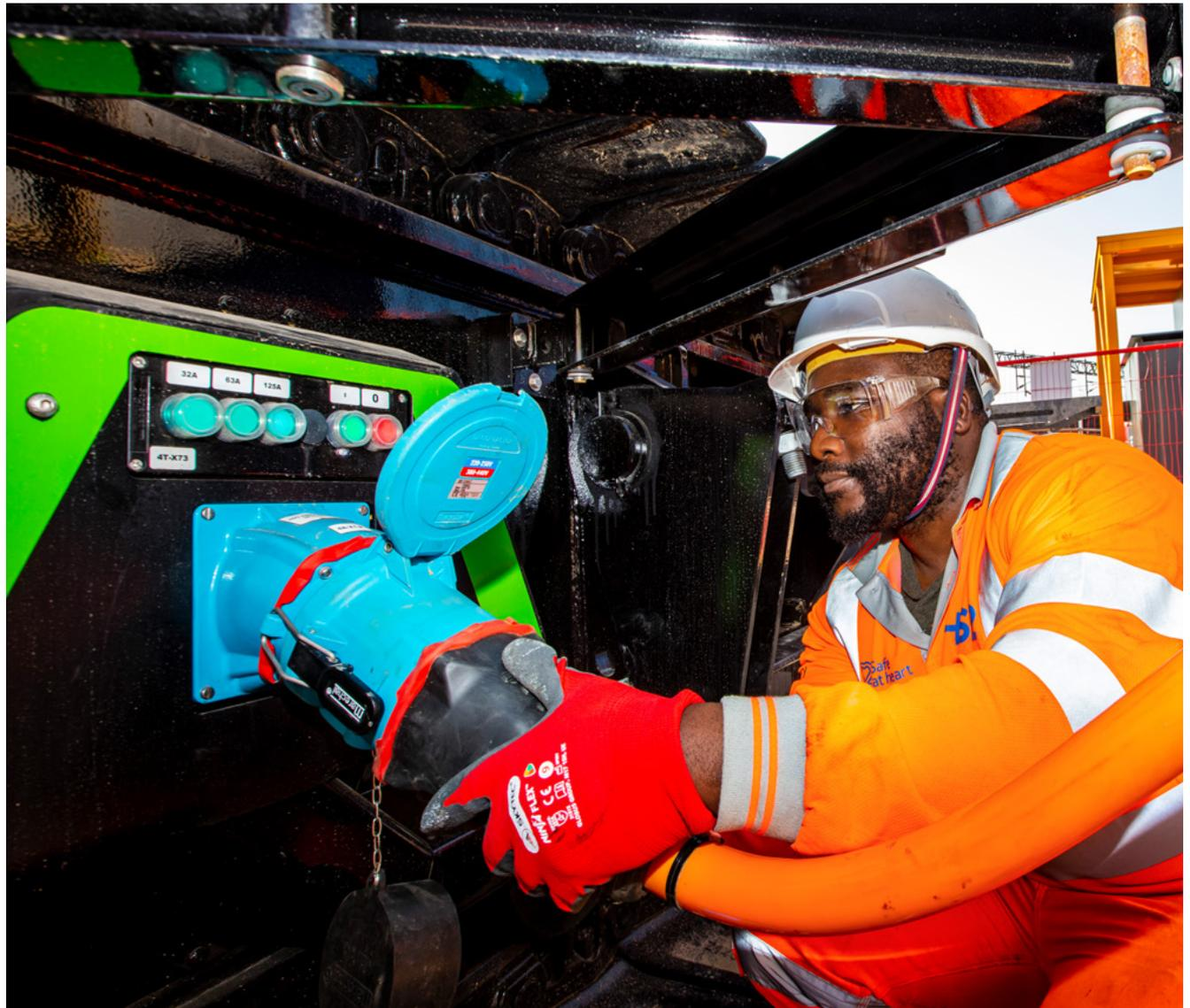
Charging an electric crane at HS2's Canterbury Road vent shaft in London.
