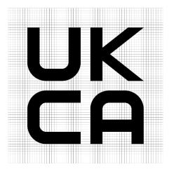
If the UK marking is reduced or enlarged according to the size of the equipment the proportions given in the above drawing must be respected. The various components of the UK marking must have substantially the same vertical dimension which may not be less than 5 mm.
