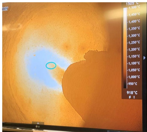
Figure 4.8: Flame shape and temperature at net zero.
