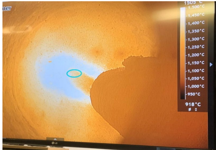
Figure 4.2: Image of the flame condition using a Thermoteknix thermal camera.
