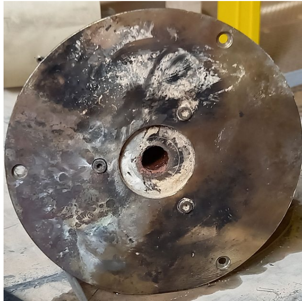
Figure 5.9: Torch tip after removal from the calciner.
