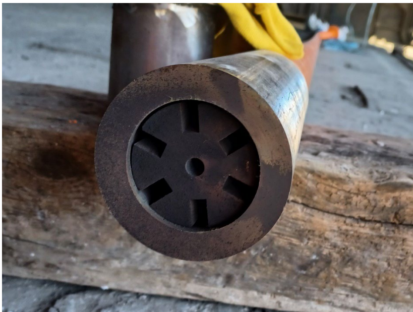
Figure 4.5: Hydrogen lance burner tip (nozzle) shown outside of the kiln.
