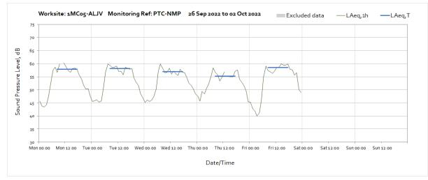
Note: Missing data from 12:00 until 13:00 on Thursday 29<sup>th</sup> September was due to the replacement of the monitoring station to allow for lab calibration of the retrieved monitoring station.
