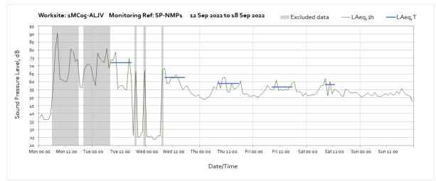
Note: High noise levels measured from Monday 12<sup>th</sup> September until Wednesday 14<sup>th</sup> September were due to a fault with the noise monitoring station and have therefore been excluded. The noise monitor was replaced on Wednesday 14<sup>th</sup> September to rectify the issue.
