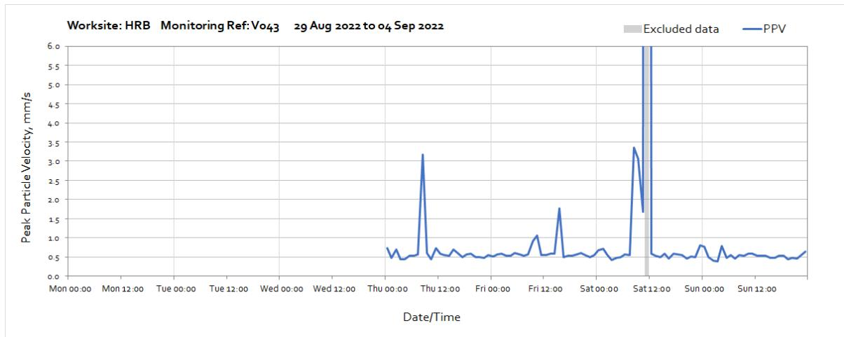
Note: High levels of vibration measured from 11:00 until 12:00 on Saturday 3<sup>rd</sup> September were due to pile mat preparation activities happening near the monitor and have therefore been excluded. Monitor is mounted on a kentledge block along the hoarding in an area of disturbed ground, vibration likely to be amplified compared to what is experienced at adjacent building. Attended monitoring booked to acquire more representative data for the receptor.
