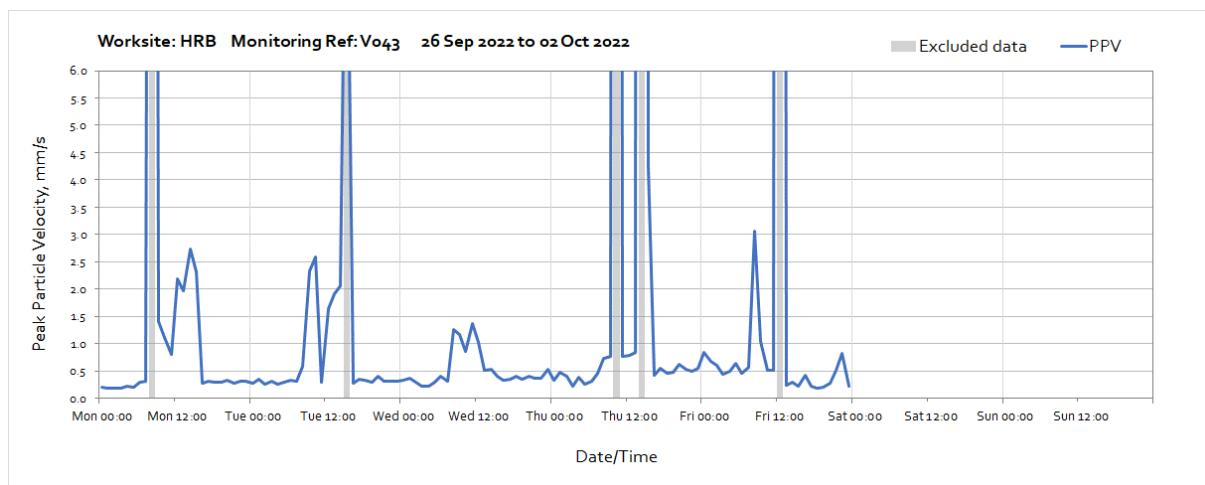
Note: High levels of vibration measured throughout the week were due to pile mat preparation activities happening near the monitor and have therefore been excluded. Monitor is mounted on a kentledge block along the hoarding in an area of disturbed ground, vibration likely to be amplified compared to what is experienced at adjacent building. Attended monitoring booked to acquire more representative data for the receptor.
