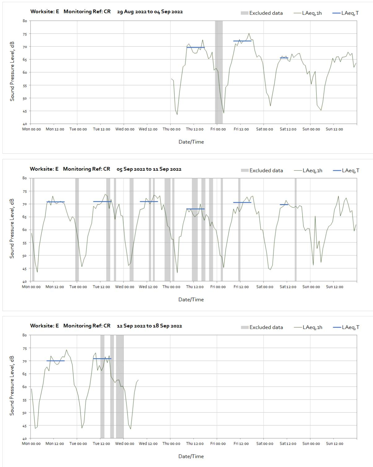
Note: Missing data from 08:00 until the end of the month was due to loss of power to the lamppost which provides power to the monitoring station. Liaison has been made with the local borough council to investigate the cause and to rectify the loss of power to the monitoring station.
