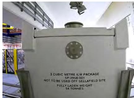
Successfully completed a test run to move 3m<sup>3</sup> boxes of nuclear waste into the new Box Encapsulation Plant Product Store Direct Import Facility. This is an important step in demonstrating the route that will be used for waste retrieved from the legacy silos.
