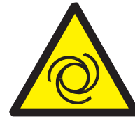
Machinery starts automatically
