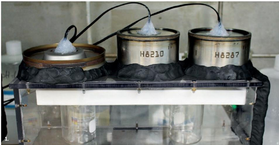
1. Experimental set up for hydrochloric acid exposure test
