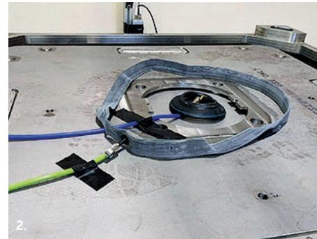
**1. Setting up the acoustic signal experiments using inner tubes inside the inner package**
