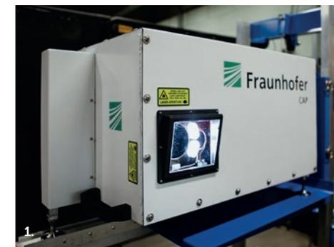
1. Hydrogen sensor for in-situ monitoring
