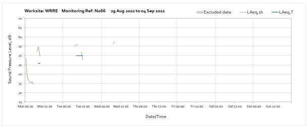
Note: Missing data throughout the week was due to loss of battery power at the monitoring station.
