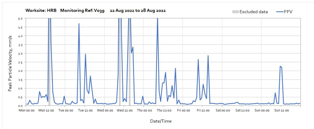
Note: High levels of vibration measured throughout the week were due to pile mat preparation activities undertaken near to the monitoring station. The monitoring station is mounted on a kentledge block along the hoarding in an area of disturbed ground, vibration is likely to be amplified compared to what is experienced at building. Attended monitoring has been booked to acquire more representative data for the receptor.
