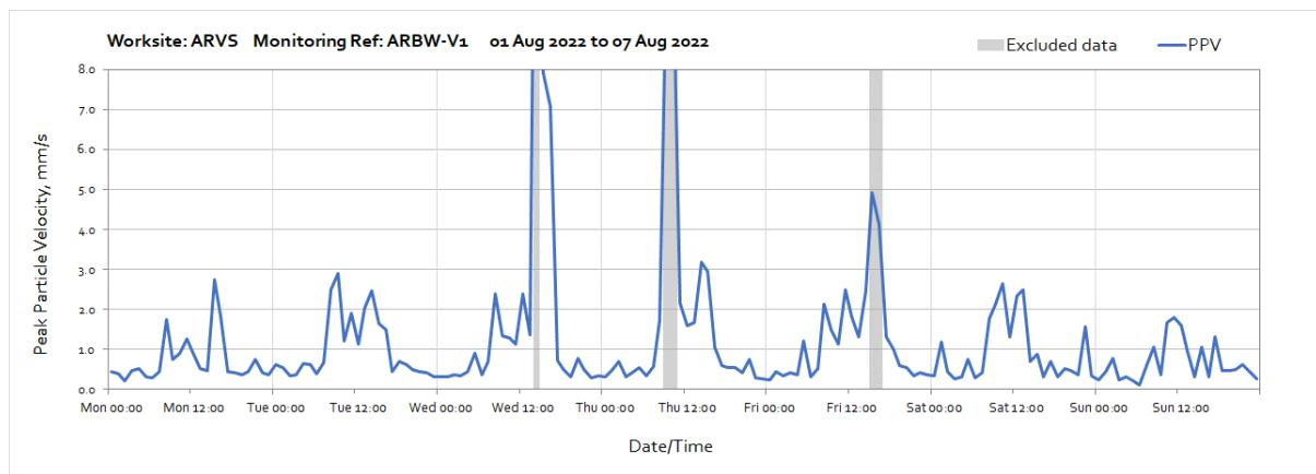
Note: High levels of vibration measured from 15:00 until 17:00 on Wednesday 3<sup>rd</sup> August were due to utilities work being undertaken in close proximity to the monitor. Vibration levels at the nearest receptor will be lower.
