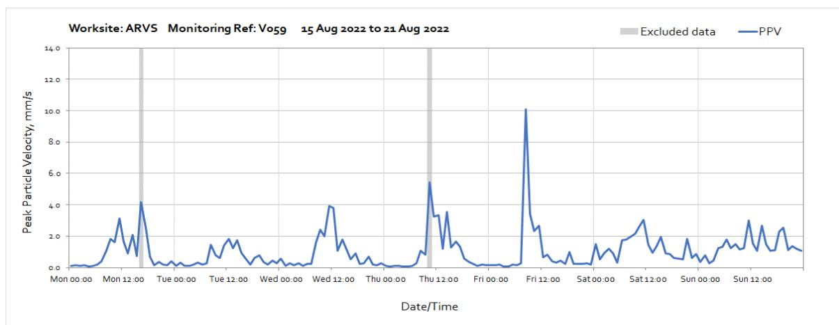
Note: High levels of vibration measured from 08:00 until 09:00 on Friday 19<sup>th</sup> August were due to utilities work being undertaken in close proximity to the monitor. Vibration levels at the nearest receptor will be lower.
