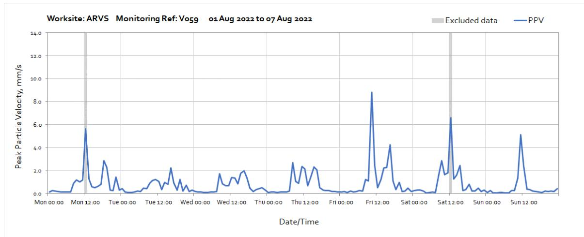
Note: High levels of vibration measured from 10:00 until 11:00 on Friday 5<sup>th</sup> August were due to utilities work being undertaken in close proximity to the monitor. Vibration levels at the nearest receptor will be lower.
