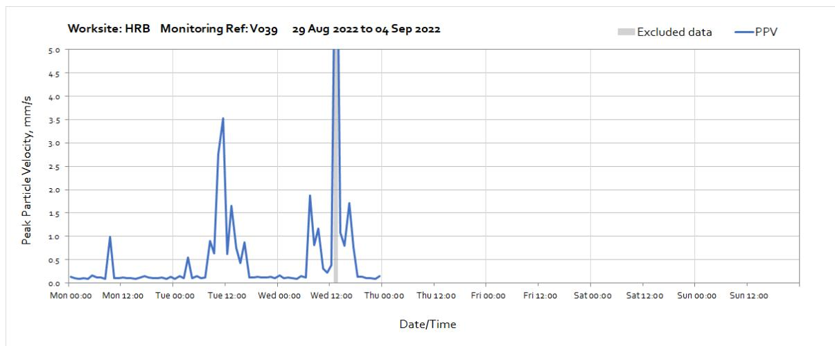
Note: High levels of vibration measured from 13:00 until 14:00 on Wednesday 31<sup>st</sup> August were due to pile mat preparation activities undertaken near to the monitoring station. The monitoring station is mounted on a kentledge block along the hoarding in an area of disturbed ground, vibration is likely to be amplified compared to what is experienced at building. Attended monitoring has been booked to acquire more representative data for the receptor.
