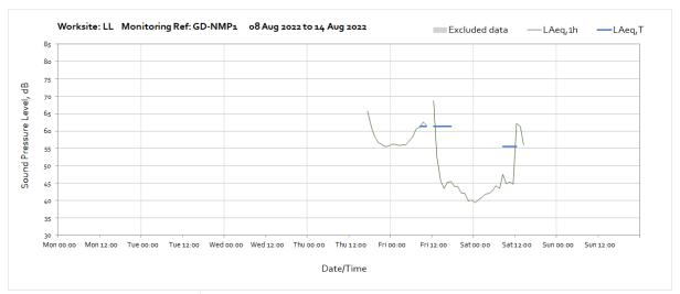
Note: Missing data until the 11<sup>th</sup> of August was due to communication cable failure. The monitor was damaged and has been replaced with a new one on the 11<sup>th</sup> of August. Missing data on the 12<sup>th</sup> at 11:00 and between the 13<sup>th</sup> of August at 15:00 and the 16<sup>th</sup> August at 12:00 was due to damage to the power supply. A replacement solar panel has been ordered.
