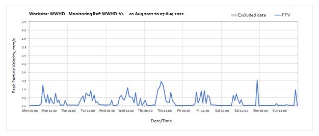
Note: High vibration levels measured throughout the week were due to movement along the haul road. The nearest sensitive receptor is 50m further away from the monitor and therefore HS2 related vibration levels will be lower at the receptor.
