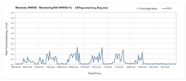
Note: High vibration levels measured throughout the week were due to plant movement along the haul road. The nearest sensitive receptor is 50m further away from the monitor and therefore HS2 related vibration levels will be lower at the receptor.
