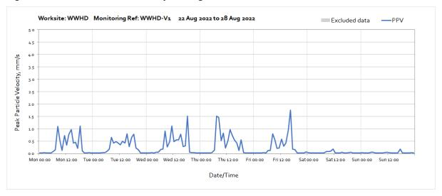
Note: High vibration levels measured throughout the week were due to loading & unloading rebar and use of roller near the monitor. The nearest sensitive receptor is 50m further away from the monitor and therefore HS2 related vibration levels will be lower at the receptor.
