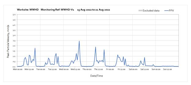
Note: High vibration levels measured throughout the week were due to ADT movement along the haul road, steel loading, use of roller near the monitor. The nearest sensitive receptor is 50m further away from the monitor and therefore HS2 vibration levels will be lower at the receptor.
