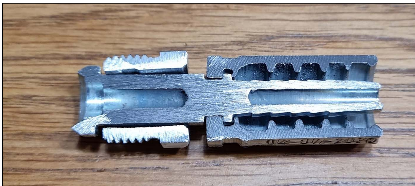
Figure 2: Section through blocked CO 2 pilot hose coupling showing incomplete bore through the stem
