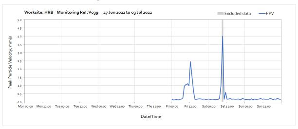
Note: High levels of vibration measured from 09:00 until 10:00 on Saturday 2<sup>nd</sup> July were due to pile mat preparation activities undertaken near to the monitoring station. The monitoring station is mounted on a kentledge block along the hoarding in an area of disturbed ground, vibration is likely to be amplified compared to what is experienced at building. Attended monitoring has been booked to acquire more representative data for the receptor.
