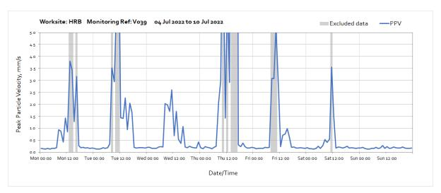
Note: High levels of vibration measured throughout the week were due to pile mat preparation activities undertaken near to the monitoring station. The monitoring station is mounted on a kentledge block along the hoarding in an area of disturbed ground, vibration is likely to be amplified compared to what is experienced at building. Attended monitoring has been booked to acquire more representative data for the receptor.
