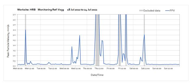
Note: High levels of vibration measured throughout the week were due to pile mat preparation activities undertaken near to the monitoring station. The monitoring station is mounted on a kentledge block along the hoarding in an area of disturbed ground, vibration is likely to be amplified compared to what is experienced at building. Attended monitoring has been booked to acquire more representative data for the receptor.
