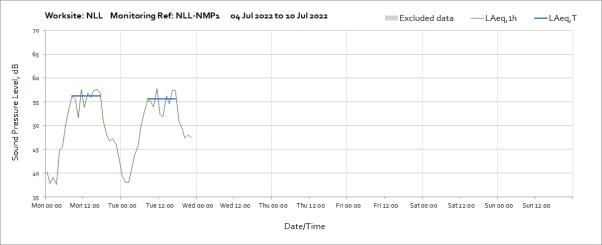
Note: Missing data from 23:00 on the  $5^{th}$  July due to severed solar panel cable, the supplier is sending a replacement.
