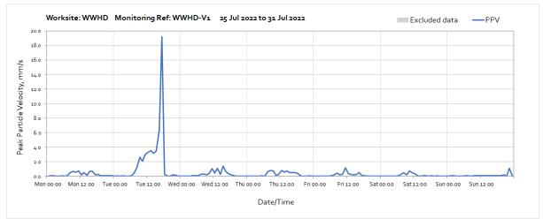
Note: High vibration levels measured throughout the week were due to digging works undertaken next to the monitoring station. The nearest sensitive receptor is 30m further away compared to the monitor and therefore HS2 vibration levels will be lower at the receptor.
