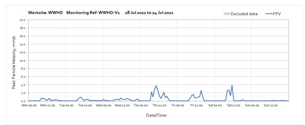
Note: High vibration levels measured throughout the week were due to earthworks and digging works undertaken next to the monitoring station. The nearest sensitive receptor is 30m further away compared to the monitor and therefore HS2 vibration levels will be lower at the receptor.
