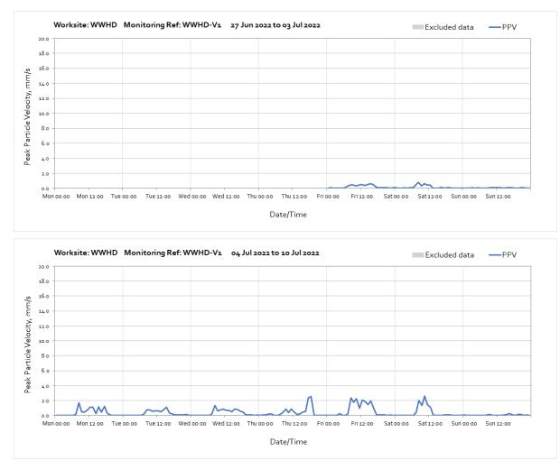
Note: High vibration levels measured throughout the week were due to digging works undertaken next to the monitoring station. The nearest sensitive receptor is 30m further away compared to the monitor and therefore HS2 vibration levels will be lower at the receptor.
