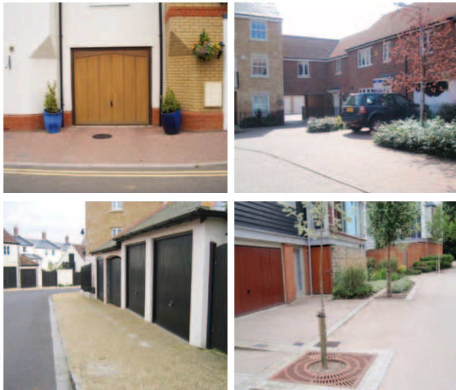
Good practice examples. Top left: Setback in excess of standard, yet with parking restrictions to prevent obstruction. Top right: Parking space clear of footway, in line with vegetation. Bottom left: Reduced setback but demarcated to show footway limit and allow room for garage door to open. Bottom right: Setback in excess of standard, yet parking can occur between dwelling and landscaping (trees), causing no obstruction to footway/carriageway
