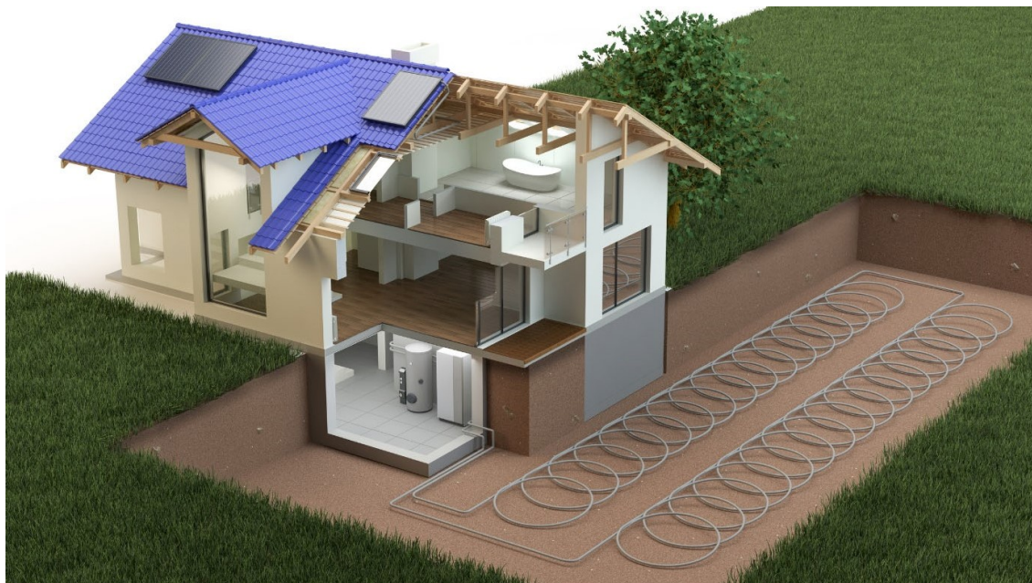
Horizontally sunk ground source heat pump
