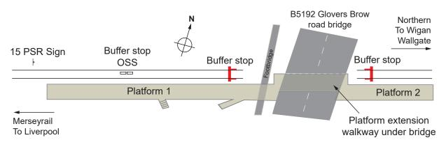
Figure 3: Diagram showing the track and station layout at Kirkby
