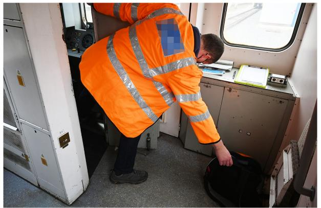
Figure 10: Photograph of a reconstruction showing how the driver could have reached his bag while maintaining pressure on the DSD pedal with his left foot
