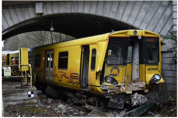
Figure 2: Photograph of the train in its final position after the collision
