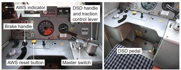
Figure 6: Photograph of the driving cab of a class 507, showing the position of the DSD and AWS controls
