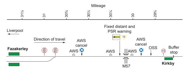
Figure 7: Schematic showing the track layout and associated infrastructure between Fazakerley and Kirkby
