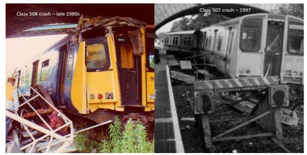
*Figure 11: Photographs of buffer stop collisions at Kirkby in a) 1987 and b) 1997 (courtesy of Network Rail)*
