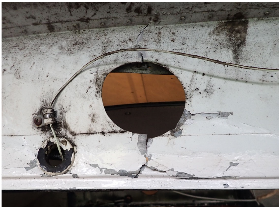
Figure 3 G-OVFM cracking of right wing root
