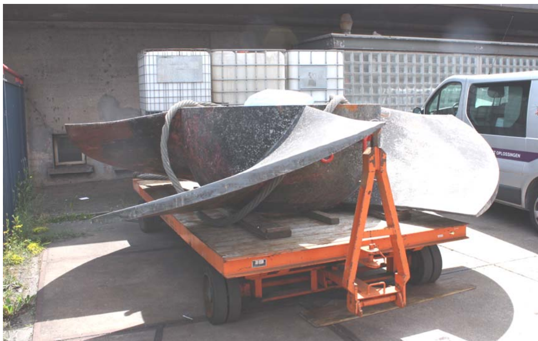
Figure F5.3. Pump impeller from one of the eight axial-flow pumps at IJmuiden, removed for maintenance.
