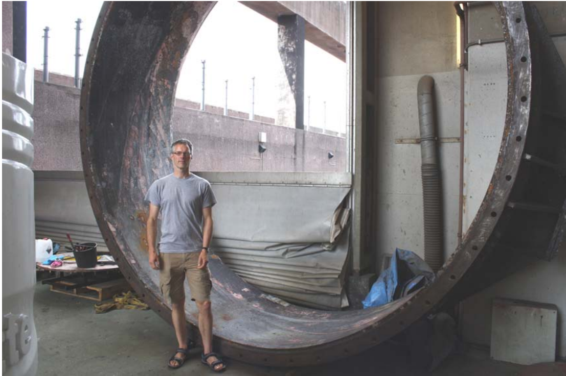
Figure F5.4. Impeller housing from one of the pumps at IJmuiden.
