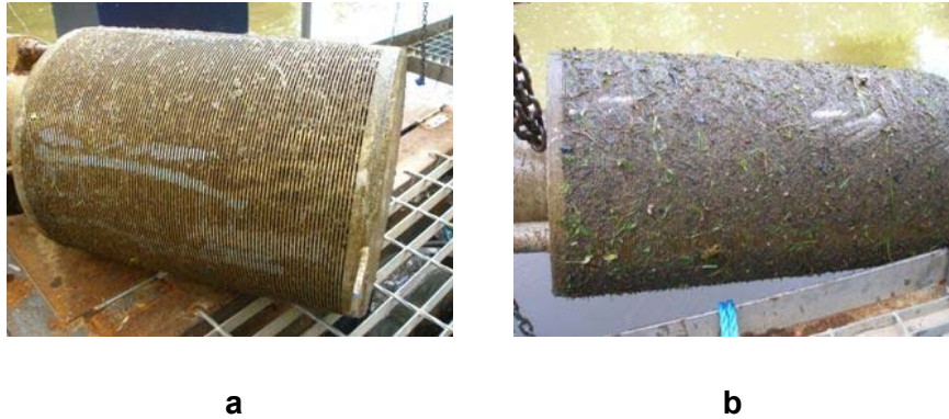
Figure 4.20 a and b: V-wire pump guard screens. Figure 4.20b shows the fouling that may occur if the screen is not fitted with an automated screen-cleaning device.
