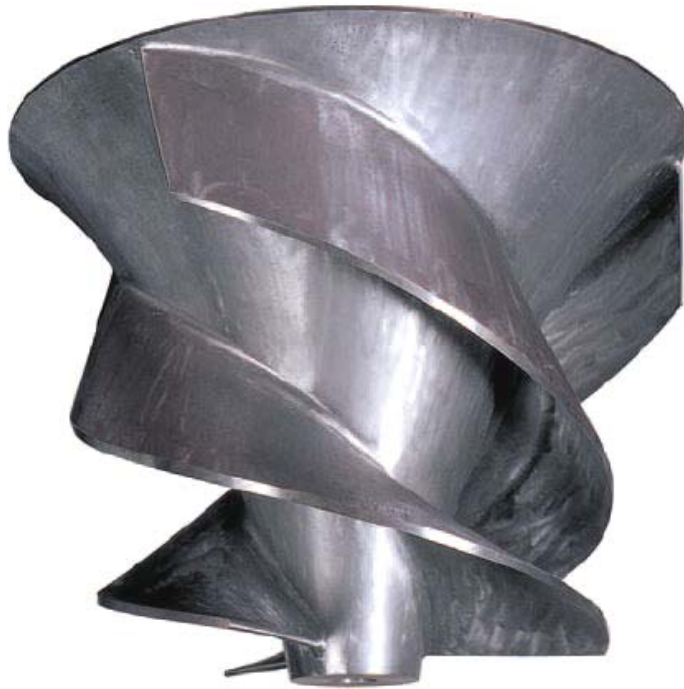
Figure F5.12. The helical runner in the Alden/NREC Advanced Turbine. This rotates in a tapered chamber with minimal gap between the outer edge of the blades and the chamber wall.
