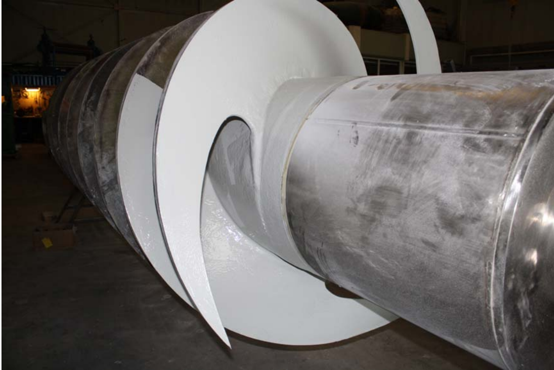
Figure F5.8. Lower end of a Fish Flow Innovations Archimedes screw pump under construction. The shape of the blade leading edge minimises collision risk and damage. The whole screw will be fitted within a rotating tube so that blade-edge gaps are eliminated. The diameter is 1.4 m, and the pumping capacity is 0.26 \text{ m}^3 \text{ s}^{-1} at 38 rpm over a head of 1.24 m.
