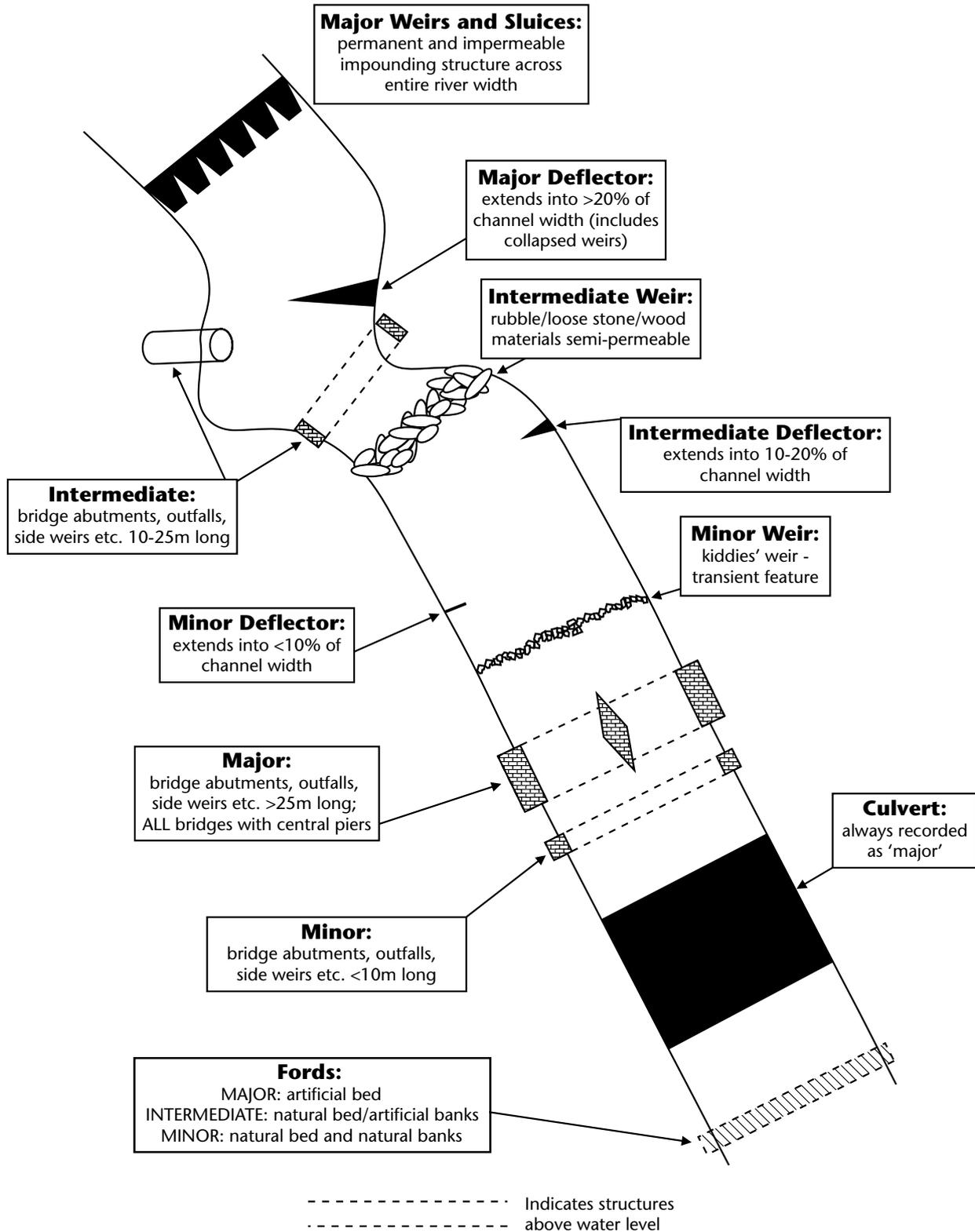
**Intermediate:** road or rail bridges **without any in-river supports**, and with bank abutments occupying 10-25m of the bank. 📷 D3c.
