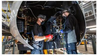
Preparing wiring inside the nose cone of a train at the Hitachi factory where some of the HS2 trains will be manufactured.
