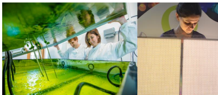
Figure 2: Current state-of-the-art APBR. 700l system using LED light tiles to internally illuminate photobioreactors.
