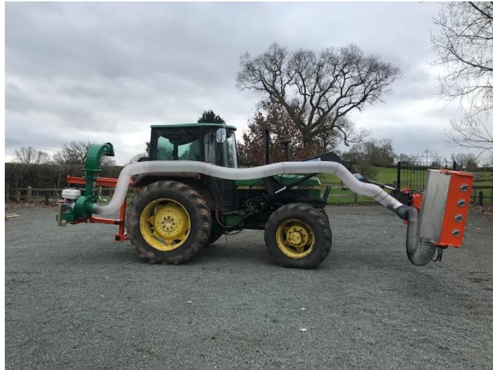
Figure 3: Small scale harvesting head and collection system mounted to tractor
