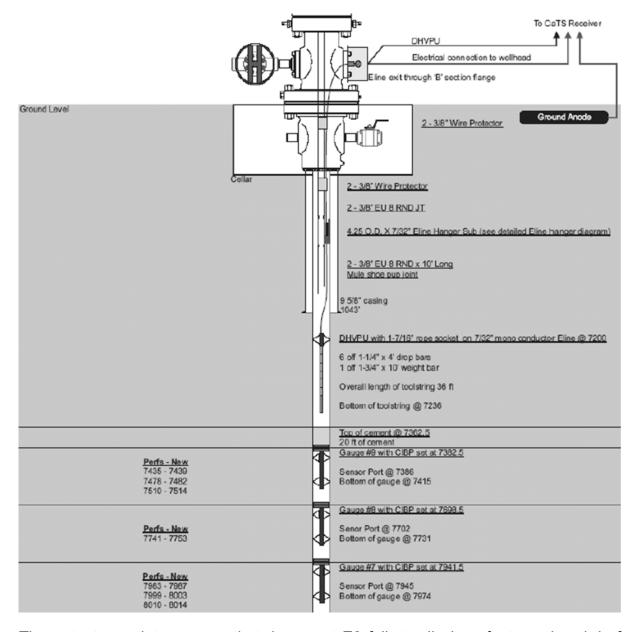
40. The patent proprietor argues that document E3 fails to disclose features I and J of claim 1. Features I and J require the connection device (i.e. the DHVPU in E3) to be
