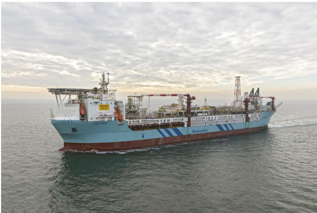
Figure 2-2 The Aoka Mizu FPSO
