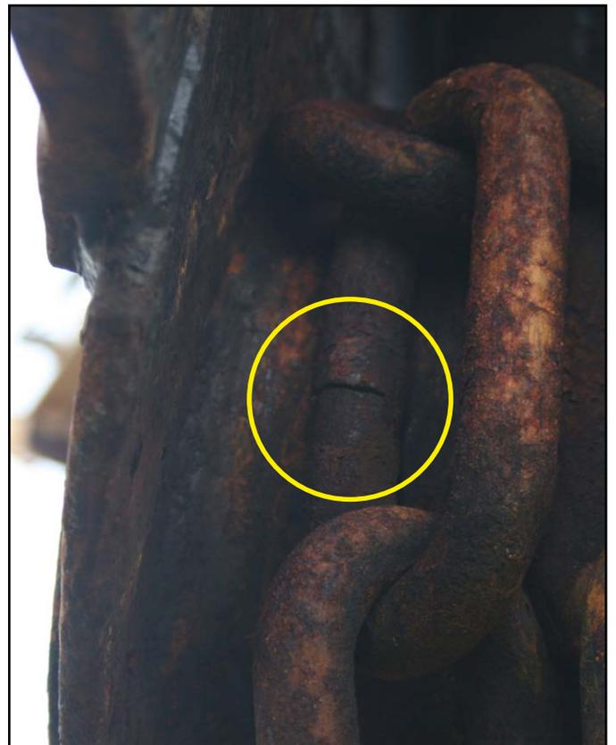
**Figure 2:** Chain fracture discovered during inspection of a quick-release mechanism on another vessel
