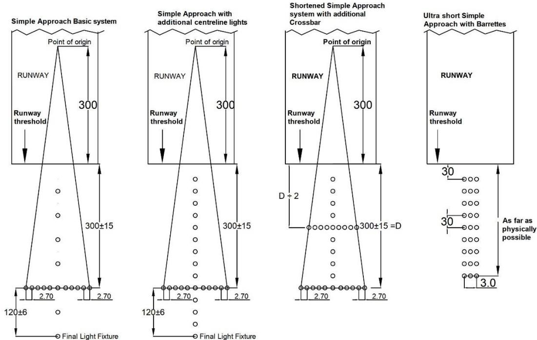
Crossbar width is to be equal to 0.05 times its distance to the Point of Origin. Having established the positions of the outer lights, the next and subsequent lights are spaced at 2.7m
