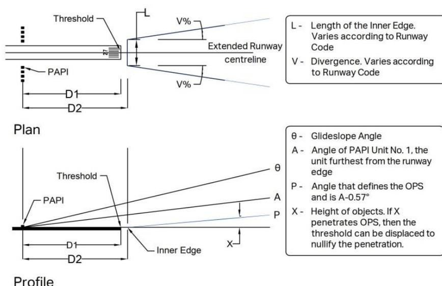
D1 = Distance from the PAPI to the Threshold, calculated to provide the required MEHT.
