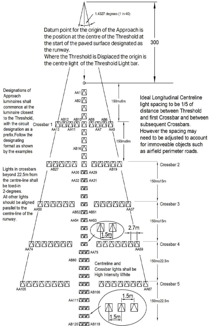
Designations of Approach luminaires shall commence at the luminaire closest to the Threshold, with the circuit designation as a prefix. Follow the designating format as shown by the examples
