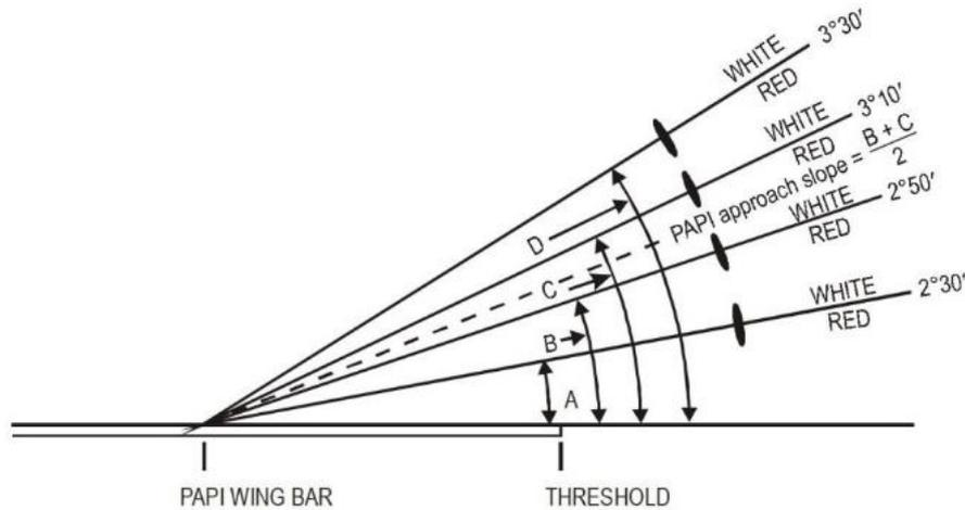
The height of the pilot's eye above the aircraft's ILS glide path/MLS antenna varies with the type of aeroplane and approach attitude. Harmonization of the PAPI signal and ILS glide path and/or MLS minimum glide path to a point closer to the threshold may be achieved by increasing the on-course sector from 20' to 30'. The setting angles for a 3° glide slope would then be 2°25', 2°45', 3°15' and 3°35'.
