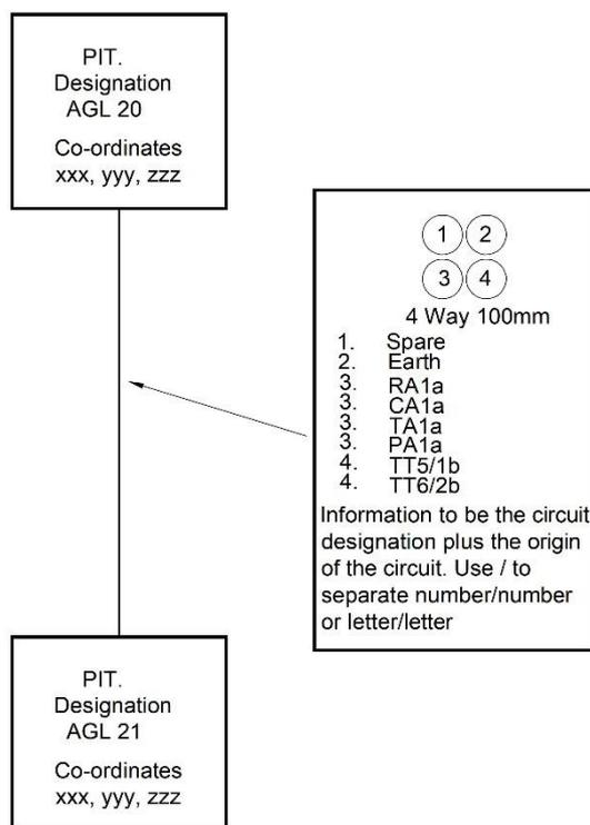
16.5.2 Each pit location shall be accompanied by a GPS reference for the centre of the pit cover accurate to within 1 metre. Referenced by xxx,yyy,zzz, where zzz is the invert level of the pit.
