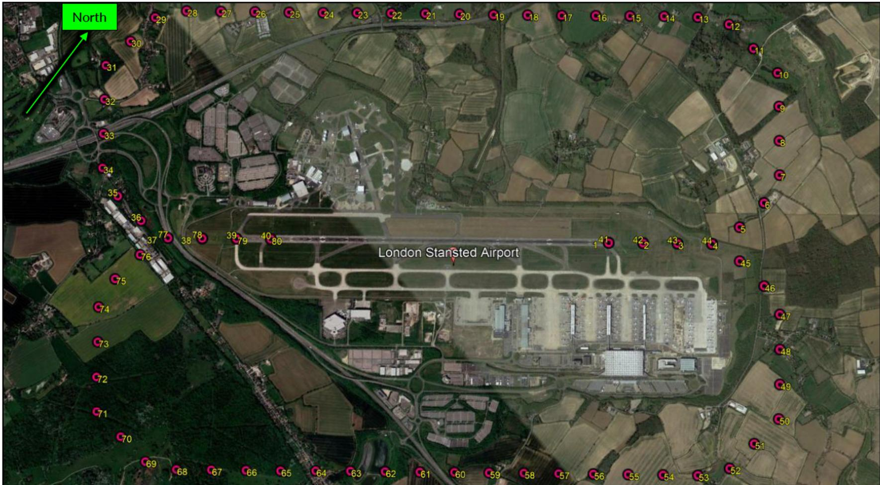
Figure 8 Assessed aircraft circuit receptors
