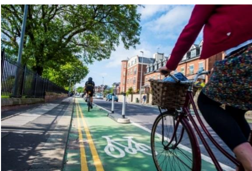
Light segregated cycle lane - with wands
