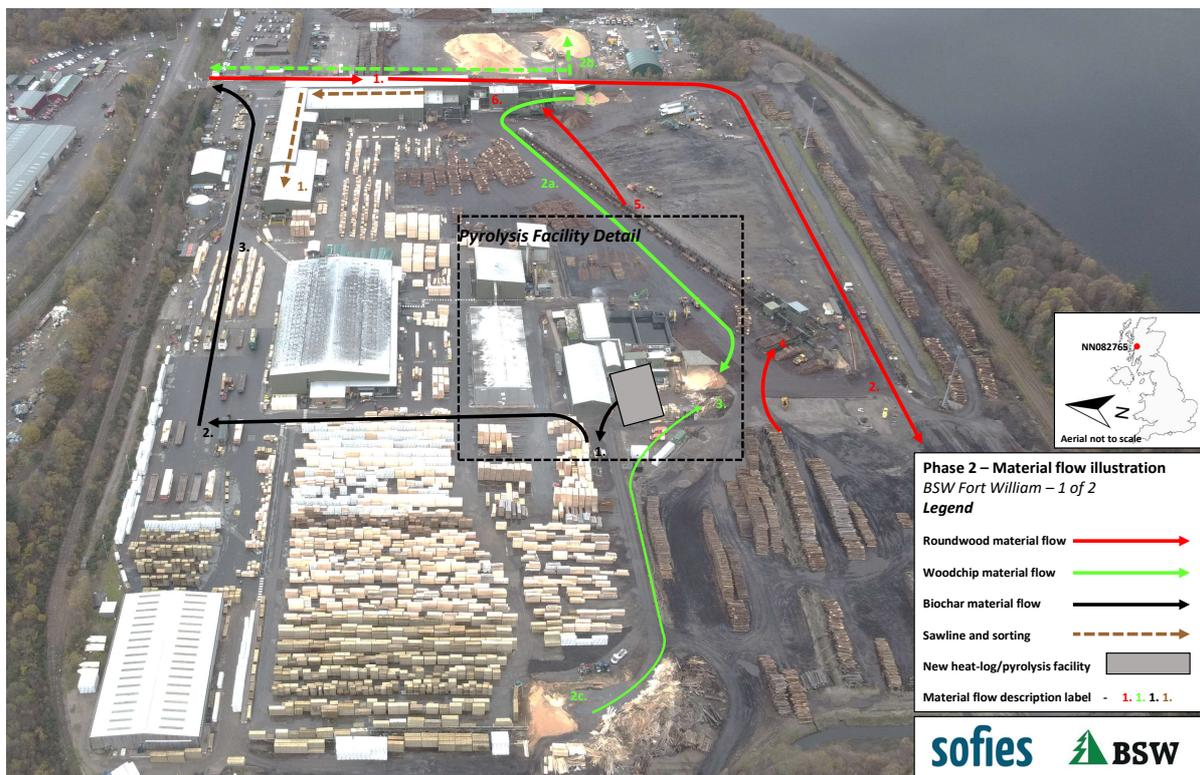
Figure 8 - Material flow diagram of the Fort William sawmill with biochar production
