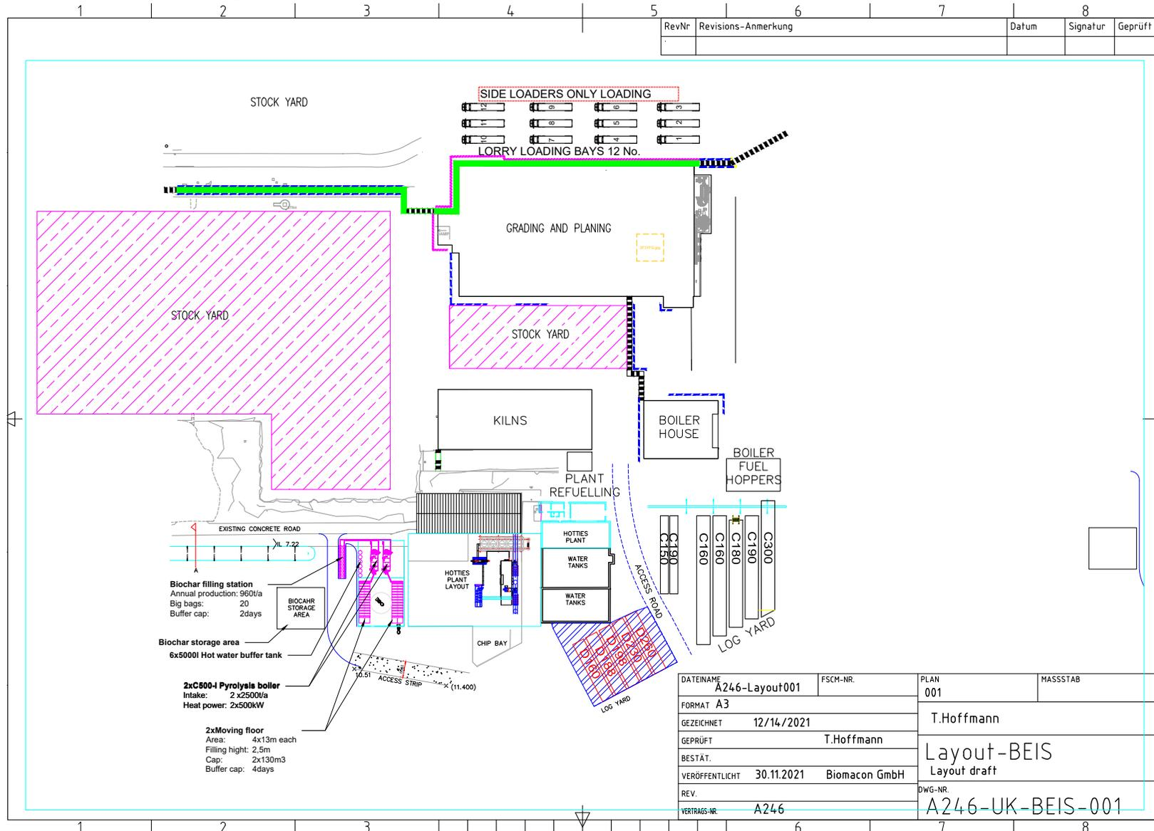
Figure 5 – Technical drawing displaying proposed Biomacon pyrolysis facility (labelled in bottom left) integrated with upgraded BSW “hotties” heatlog production line. Flexible biochar production facility comprises of two biomacon c-500i units and accompanying moving floor feed intake systems and extraction/packing systems.
