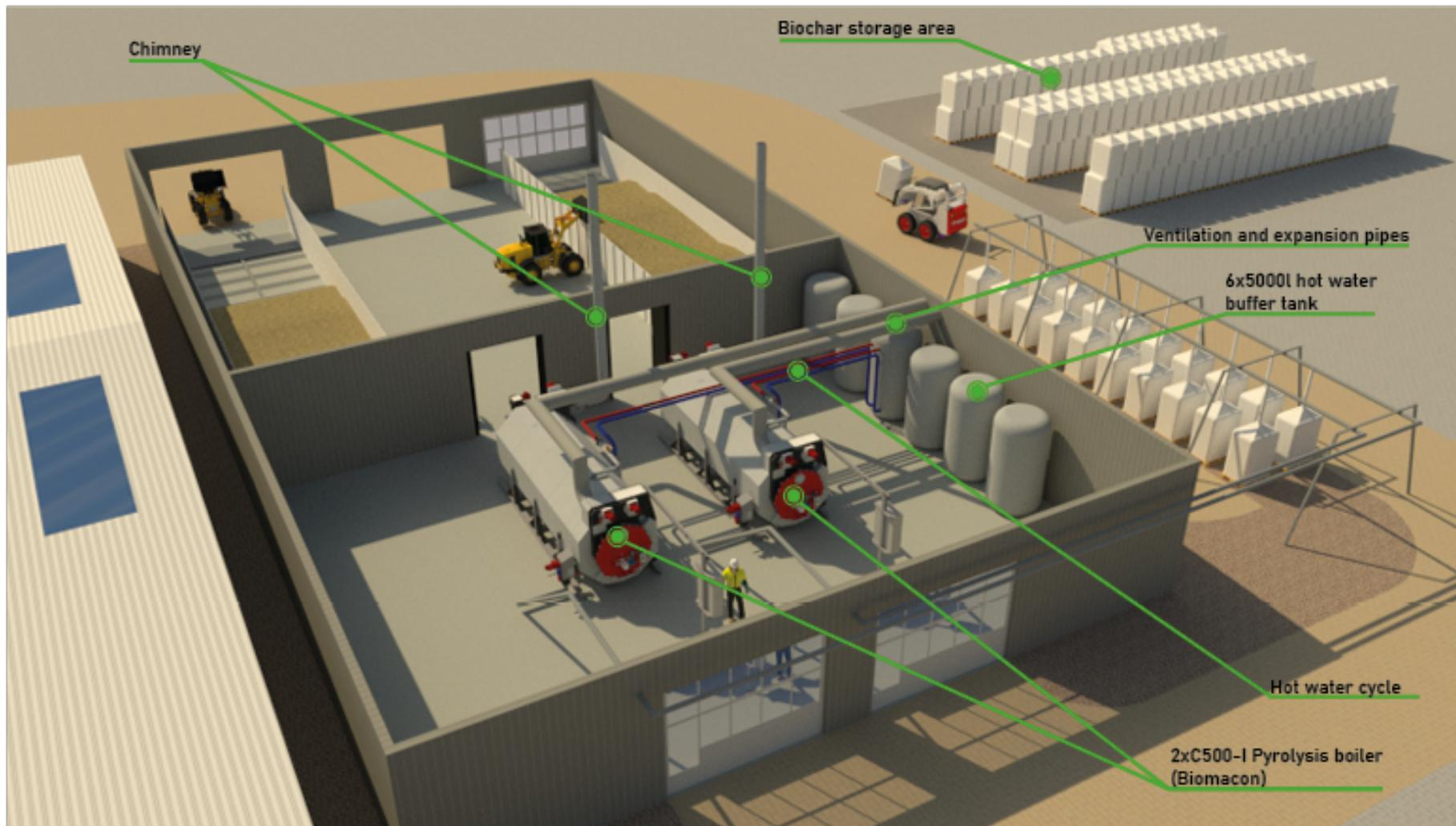
Figure 6 – 3D rendered visualisation of two side by side Biomacon C500I units at BSW Fort William. Heat will be transferred from hot water buffer tanks to BSW heat sinks (both in woodchip and timber drying processes).
