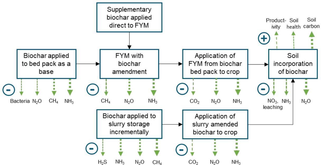
Figure 2 - Illustrative biochar scenario in manure management systems in dairy farming showing key stages in manure management systems (slurry and farmyard manure (FYM)), with point of application of biochar. Potential benefits of biochar compared with conventional manure management systems are outlined by green arrows (upward arrows showing an increase and downwards arrows a decrease, arrow thickness indicates relative extent of benefit at each stage).
