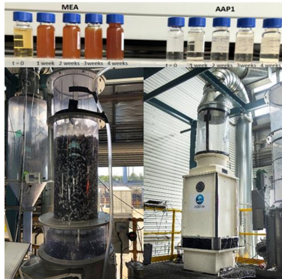
Figure 1: CSIRO TRL4 DAC system development showing comparison of absorption liquid degradation against conventional MEA (top) and different types of absorbers tested (bottom)
