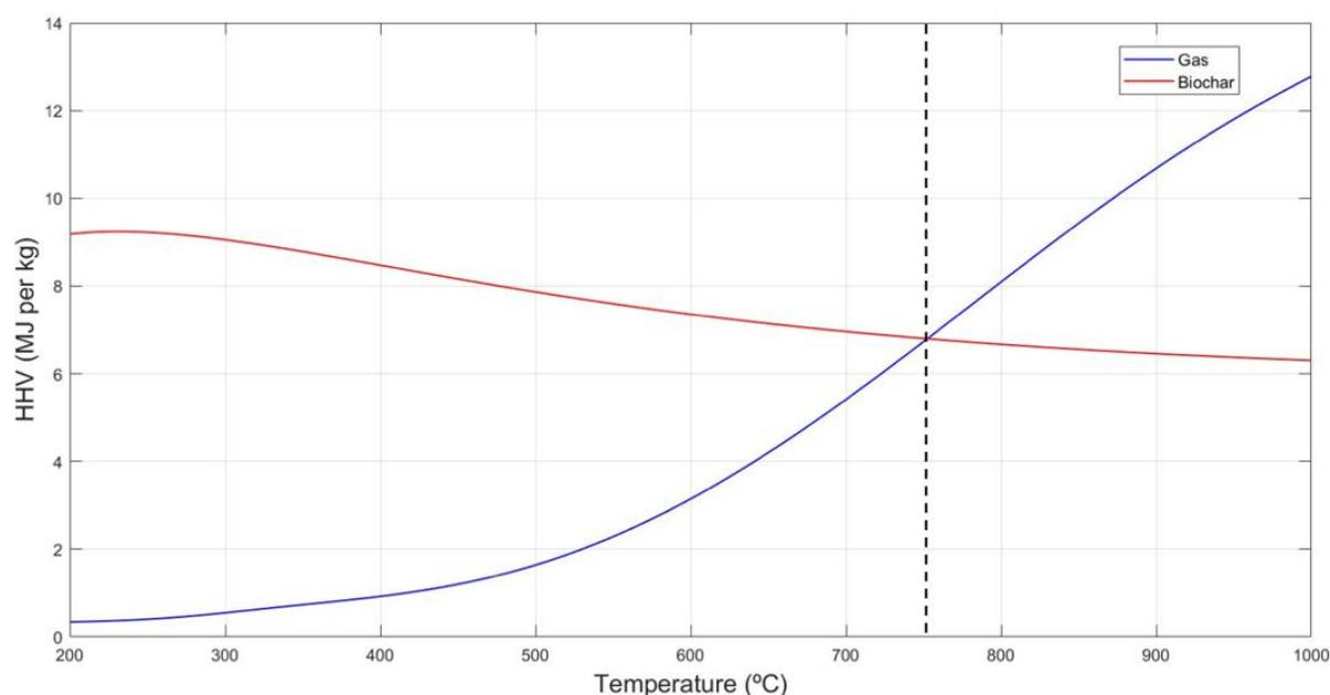
**Figure 2.2.1 Pyrolysis model - Energy outcome (Gas & Biochar) vs temperature (Experimental research by UoL)**
