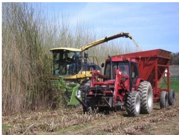
Figure 2.1.2 Forage harvester with hydraulic driven willow cutting head (photo by Lawrence Abrahamson)
